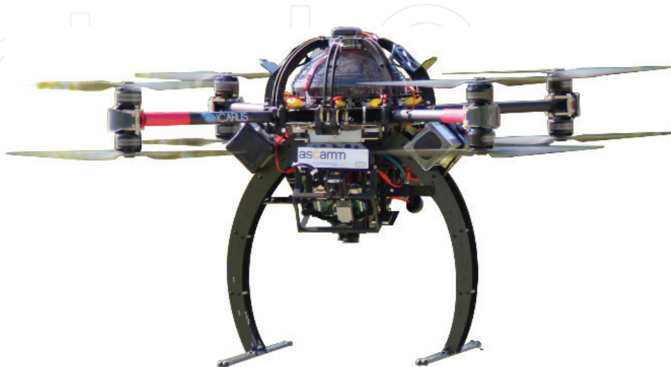
Figure 7. The Eurecat coaxial-quadrotor with the camera payload (source: ICARUS consortium).
