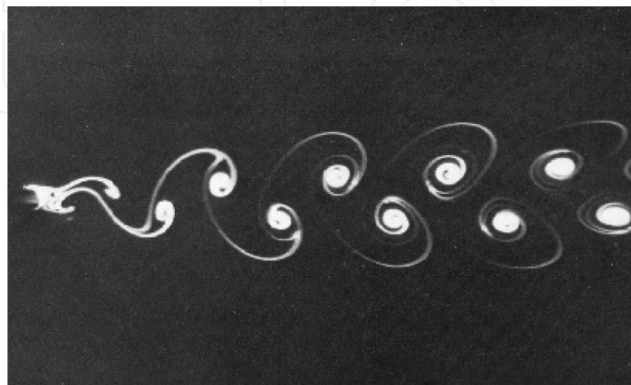
Figure 2. Von Karman streets behind a cylinder in a nonrotating 2D flow for Re = 140 , fluorescein visualization, picture taken from [3].
