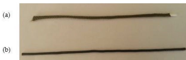
Figure 17. (a) Hybrid yarn before heating (b) Hybrid yarn after heating.
