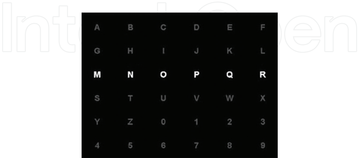
Figure 3. The row-column (RC) paradigm. One row (MNOPQR) is flashing.
