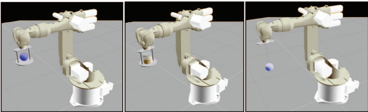
Figure 2. Three problem-scenarios in evaluation. Minimizing of shear forces (a), liquid sloshing (b) and sway oscillations (c)
