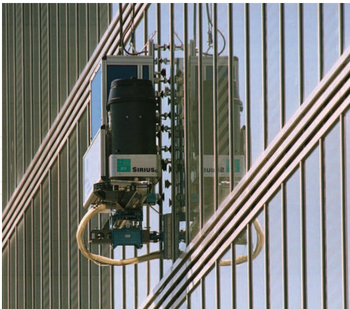
Fig. 2. SIRIUSC – Automatic Facade Cleaning System (Fraunhofer FhG, Dornier Technologie)
