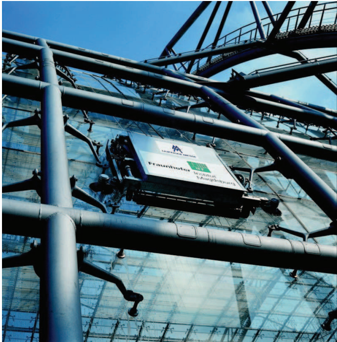
Fig. 1. Automatic Facade Cleaning System for the Vaulted Glass Hall of the Leipzig Trade Fair ( Fraunhofer FhG )
