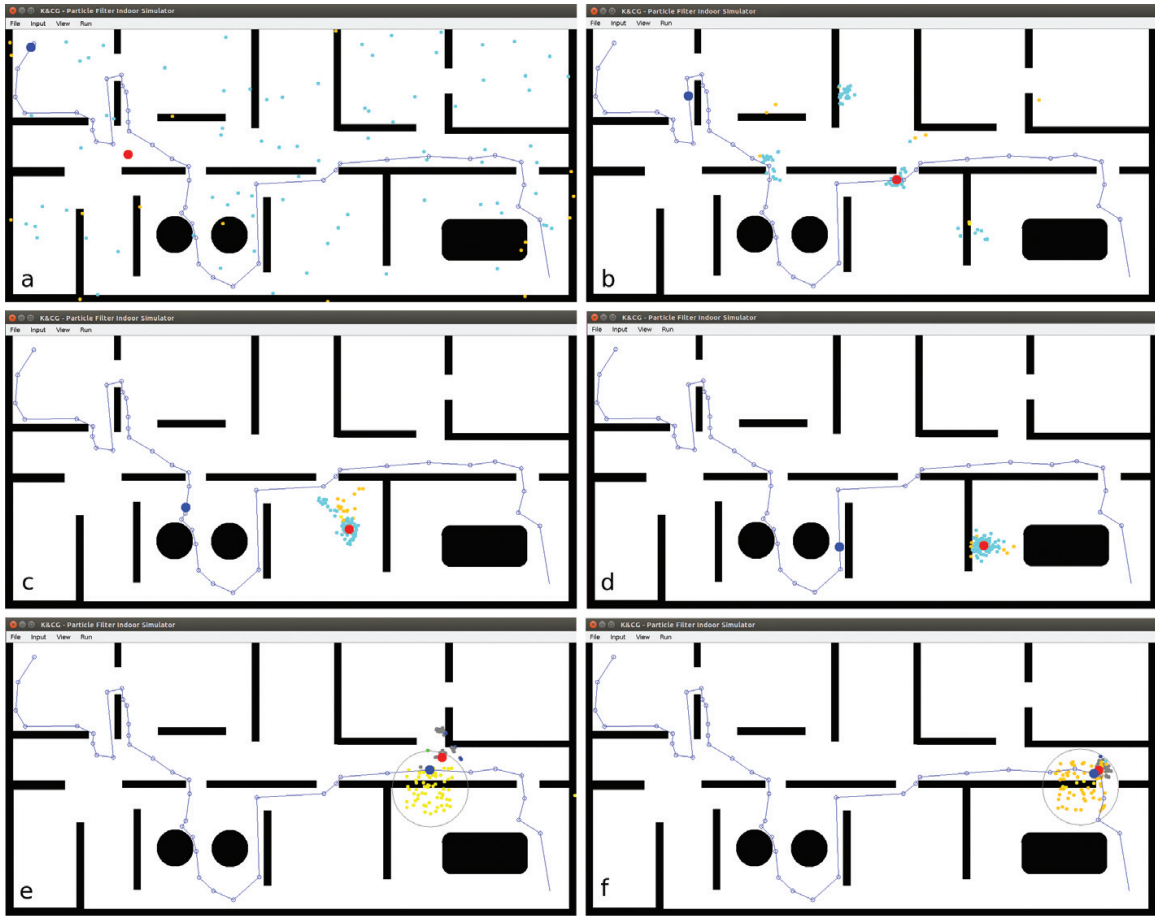
Figure 5. Particle filter in action: 100 particles were randomly located in the building (a). No RF positioning service is leading to a wrong converges (b–d), due to undersampling—the number of particles is too low. Using RF positioning (e and f), the correct position was found.
