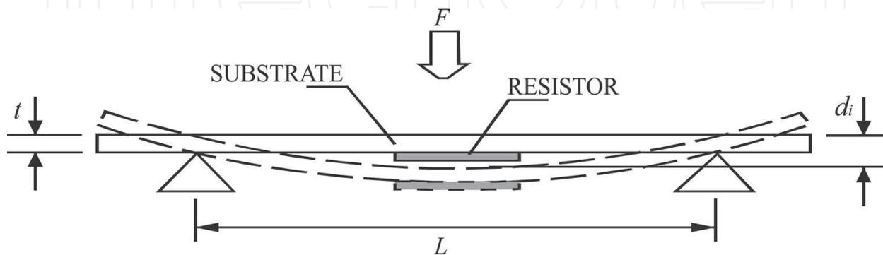
**Figure 1.** Schematic presentation of mechanically strained thick-film resistor.
