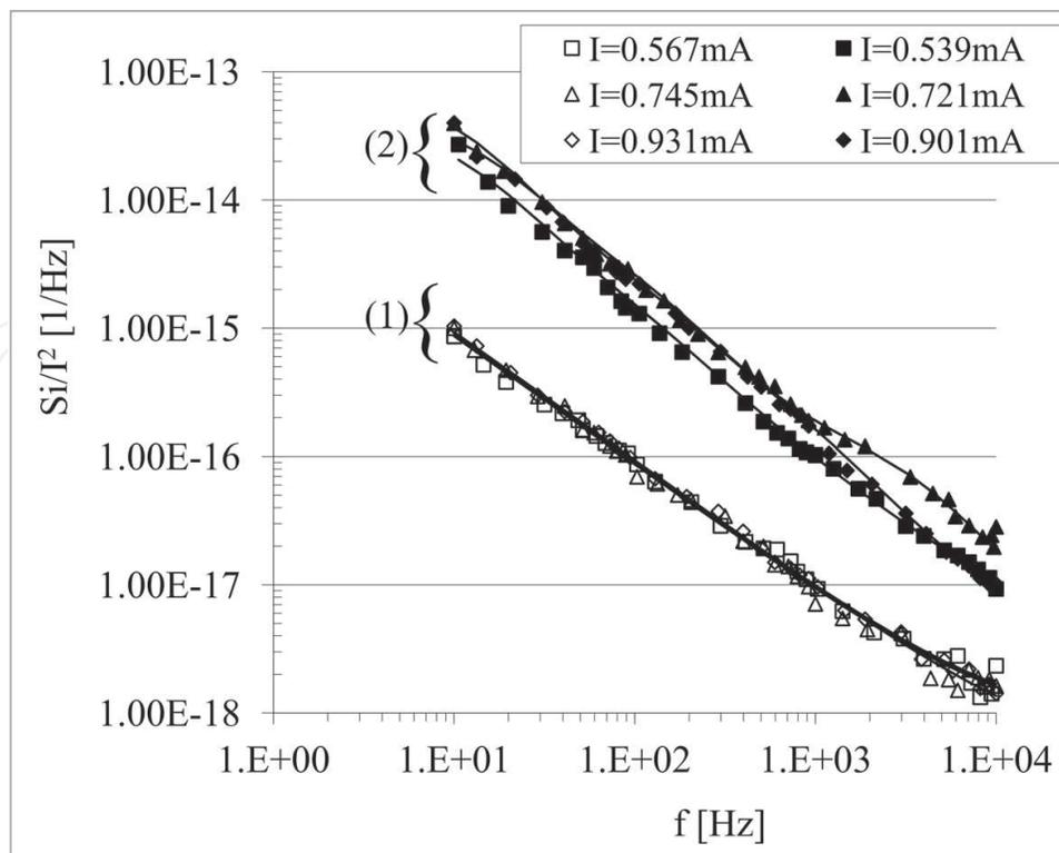
**Figure 4.** Experimental results for normalized current noise spectra before (1) and after (2) high voltage pulse stressing (multiple series of 10 pulses with increasing amplitudes) for 10 kΩ/sq thick-film resistor (full lines, fitting results) [21].
