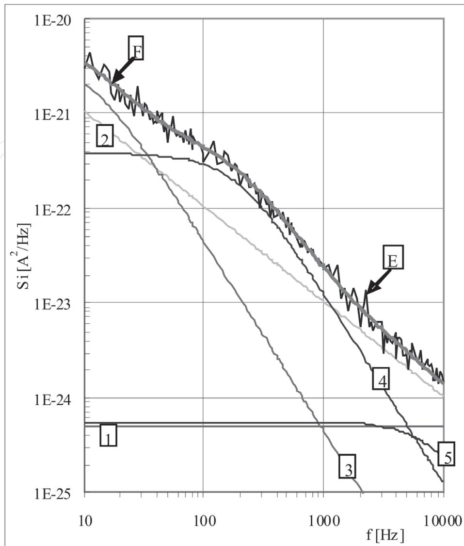
**Figure 12.** Experimental results (*E*) for current noise spectrum and fitting results (*F*) according to Eq. (4) for curve (4) in **Figure 8** with contributions of different kinds of noise sources in the total current noise spectrum (1—thermal current noise, 2— $1/f$  noise, 3, 4, 5—noise spectra of the Lorentzian shape) [16].
