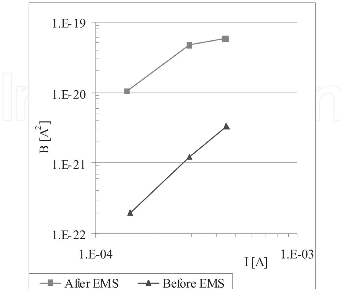
**Figure 13.**  $1/f$  noise parameter  $B_0$  before and after simultaneous mechanical and electrical straining of 10 k $\Omega$ /sq thick-film resistors (resistor width:  $w = 1$  mm, length:  $l = 4$  mm) [16].
