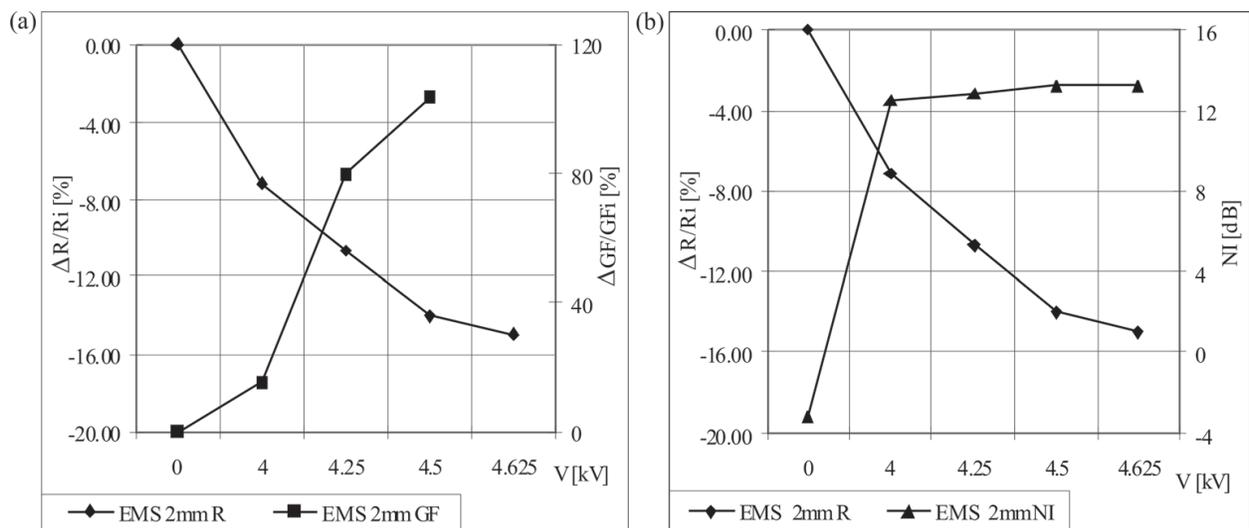
**Figure 10.** Experimental results for relative resistance, gauge factor changes (a) and noise index (b) for simultaneously mechanically and electrically strained (10 pulses per series) 100 kΩ/sq thick-film resistors (resistor width:  $w = 1$  mm, length:  $l = 2$  mm) [16].
