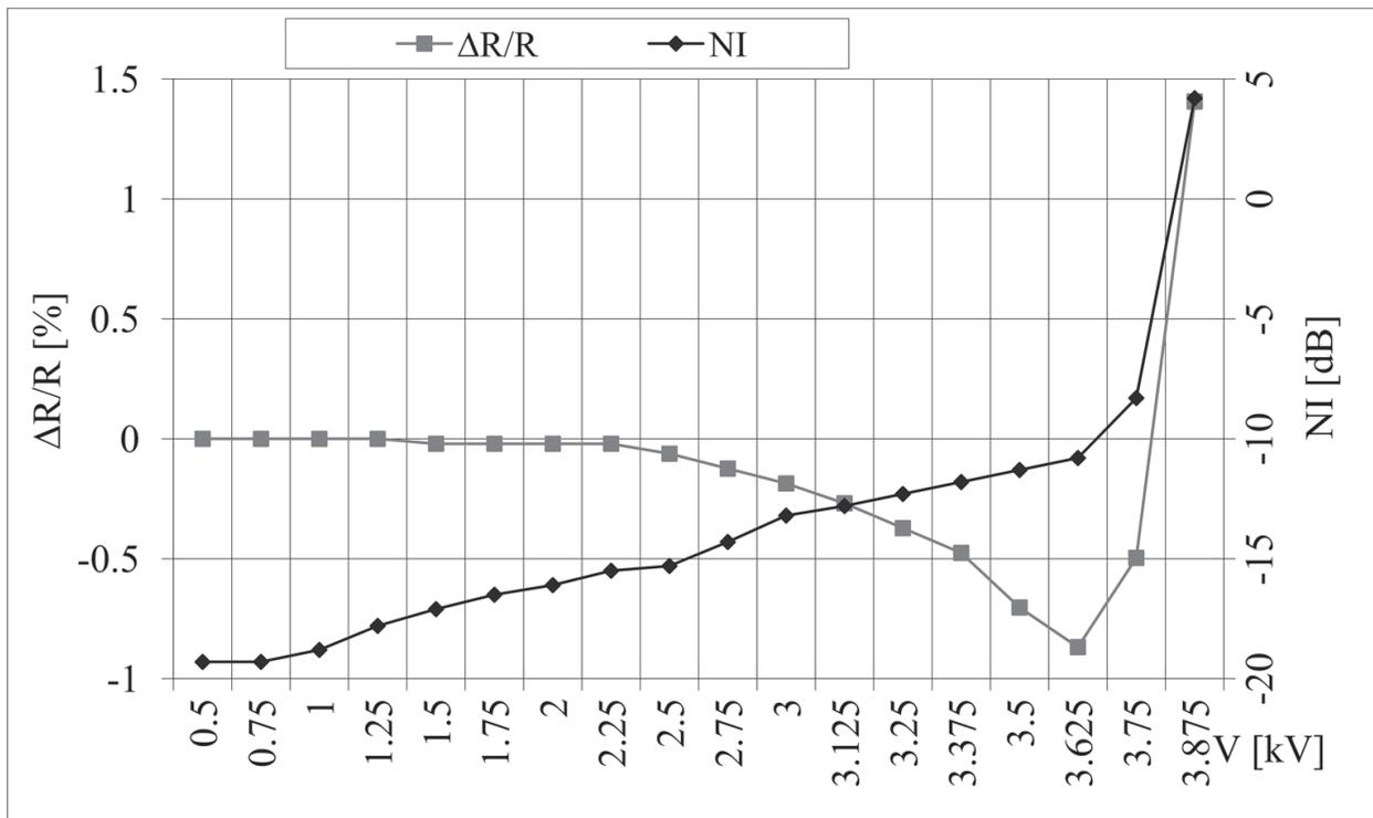
**Figure 3.** Experimental results for relative resistance and noise index changes during high voltage pulse stressing of 10 kΩ/sq thick-film resistor using multiple series of 10 pulses with increasing amplitudes (resistor width:  $w = 1$  mm, length:  $l = 3$  mm) [21].
