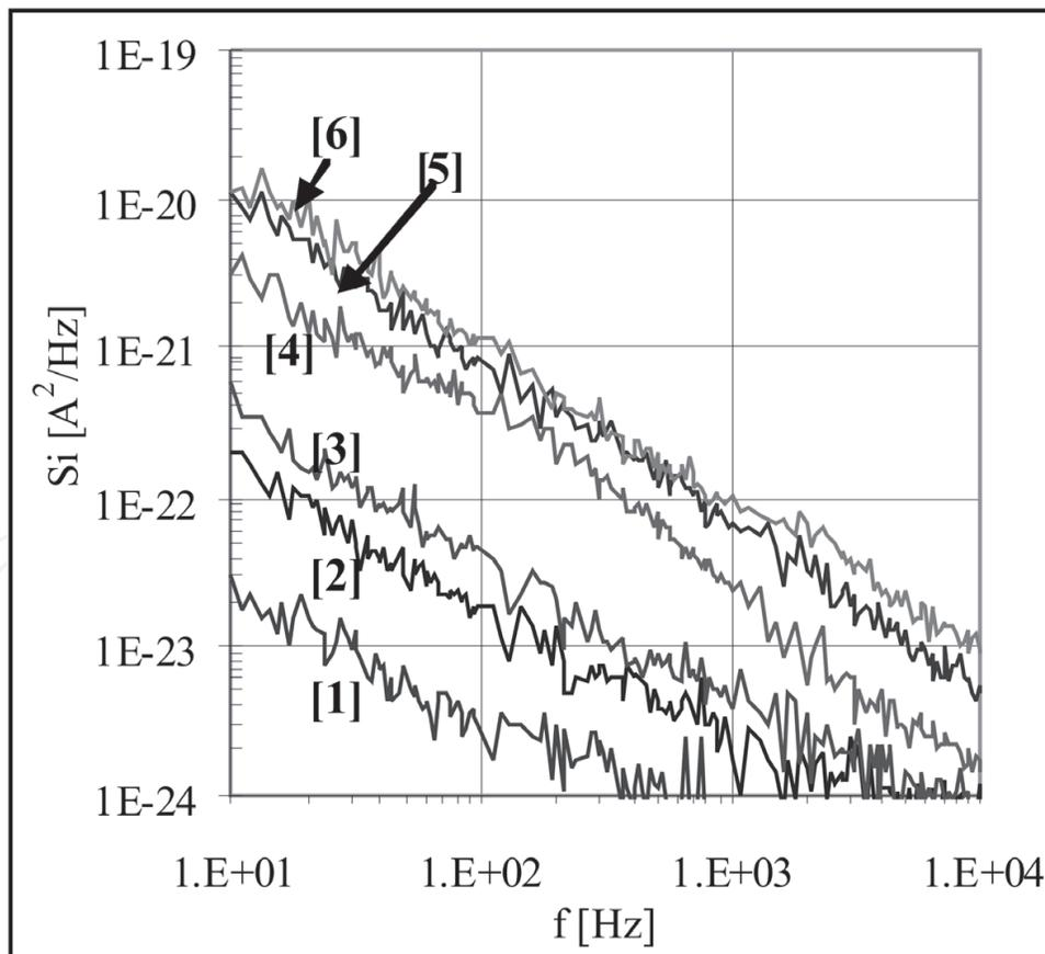
**Figure 11.** Experimental results for current noise spectrum before (1— $I = 0.1488$  mA, 2— $I = 0.2925$  mA, 3— $I = 0.4452$  mA) and after (4— $I = 0.1435$  mA, 5— $I = 0.2917$  mA, 6— $I = 0.4424$  mA) simultaneous mechanical and electrical straining of 10 k $\Omega$ /sq thick-film resistors [16].
