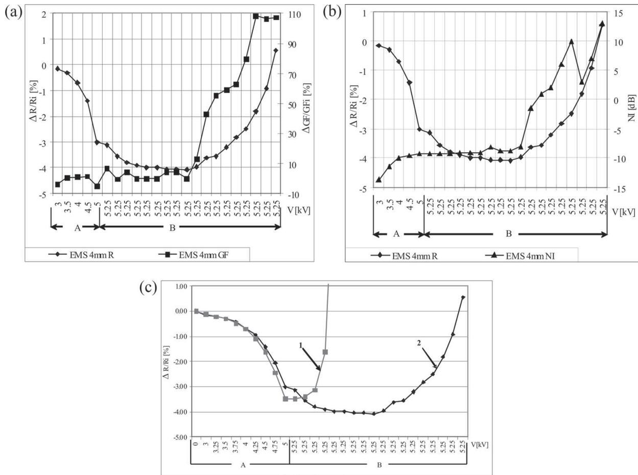
**Figure 9.** Experimentally obtained results for relative resistance, gauge factor changes (a) and noise index (b) for thick resistive films subjected to simultaneous impact of mechanical and electrical straining along with summary plot of relative resistance change (c) for electrically (1) and simultaneously mechanically and electrically strained (2) 10 kΩ/sq thick-film resistors (A—10 pulses per series, B—single pulses, resistor width:  $w = 1$  mm, length:  $l = 4$  mm) [16].
