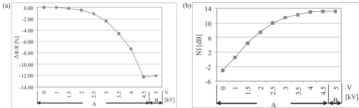
**Figure 7.** Experimental results. (A) Multiple series of 10 pulses with increasing amplitudes, (B) single pulses of the critical amplitude for relative resistance (a) and noise index (b) changes during high-voltage pulse stressing of 100 k $\Omega$ /sq thick-film resistors (resistor width:  $w = 1$  mm, length:  $l = 3$  mm) [21].
