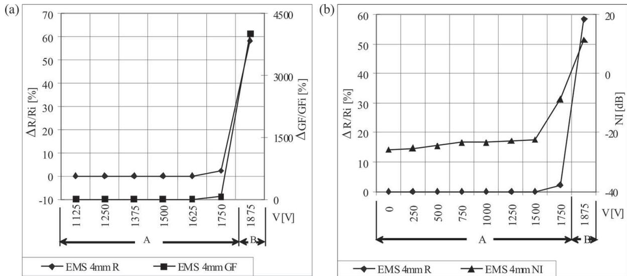
**Figure 8.** Experimental results for relative resistance, gauge factor changes (a) and noise index (b) for simultaneously mechanically and electrically strained 1 kΩ/sq thick-film resistors (resistor width:  $w = 1$  mm, length:  $l = 4$  mm) [16].
