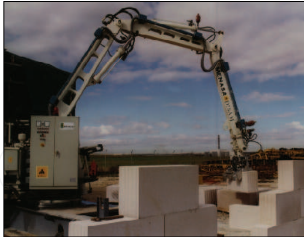
Fig. 9. ROCCO project brick assembly robot
