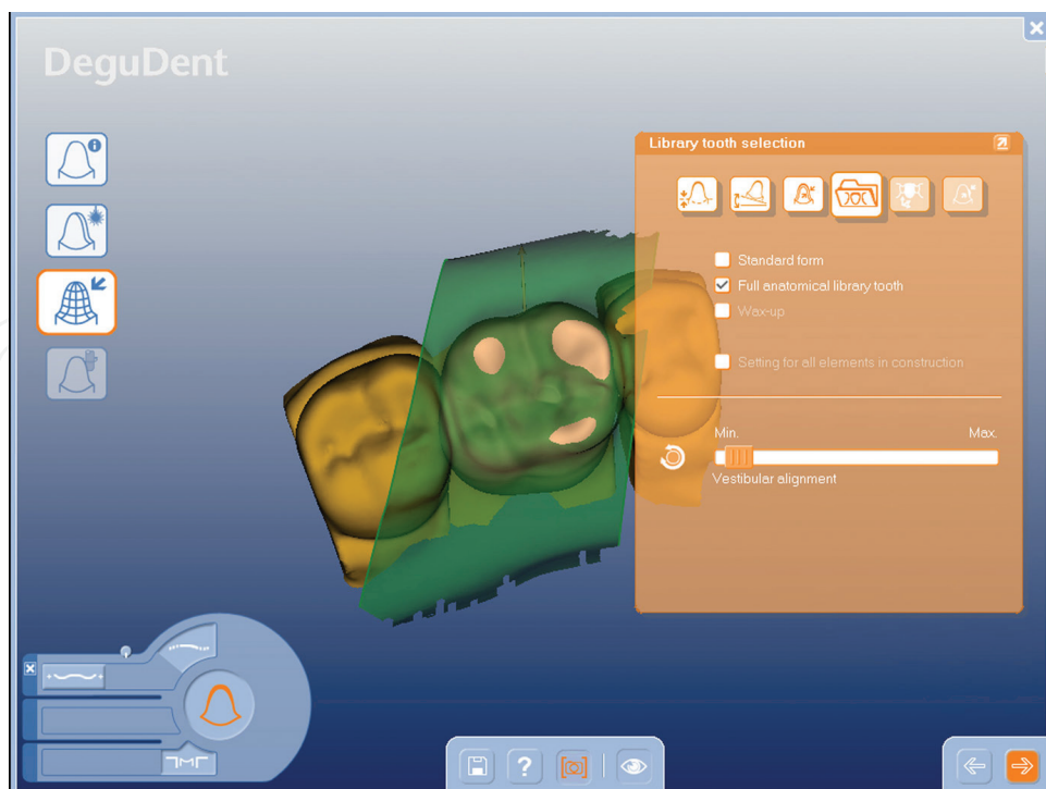
Figure 5. Zirconia anatomical framework design.
