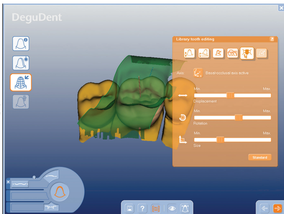
Figure 6. Zirconia anatomical framework design after optimization of the contact points with the adjacent teeth and antagonists.
