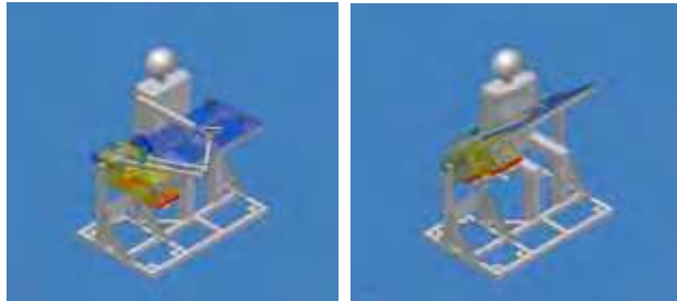
Fig. 23. Quasi-3-DOF rehabilitation system “PLEMO”: Horizontal state (left) and slanted state (right).
