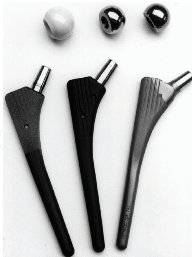
Figure 17. Carbon fiber-reinforced thermoplastic hip prosthesis, with and without hydroxyapatite coating, shown alongside conventional titanium equivalent [108].
