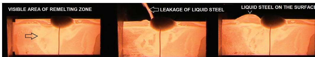
Figure 2. The view of the sample at the selected physical simulation stages (S355 grade steel).
