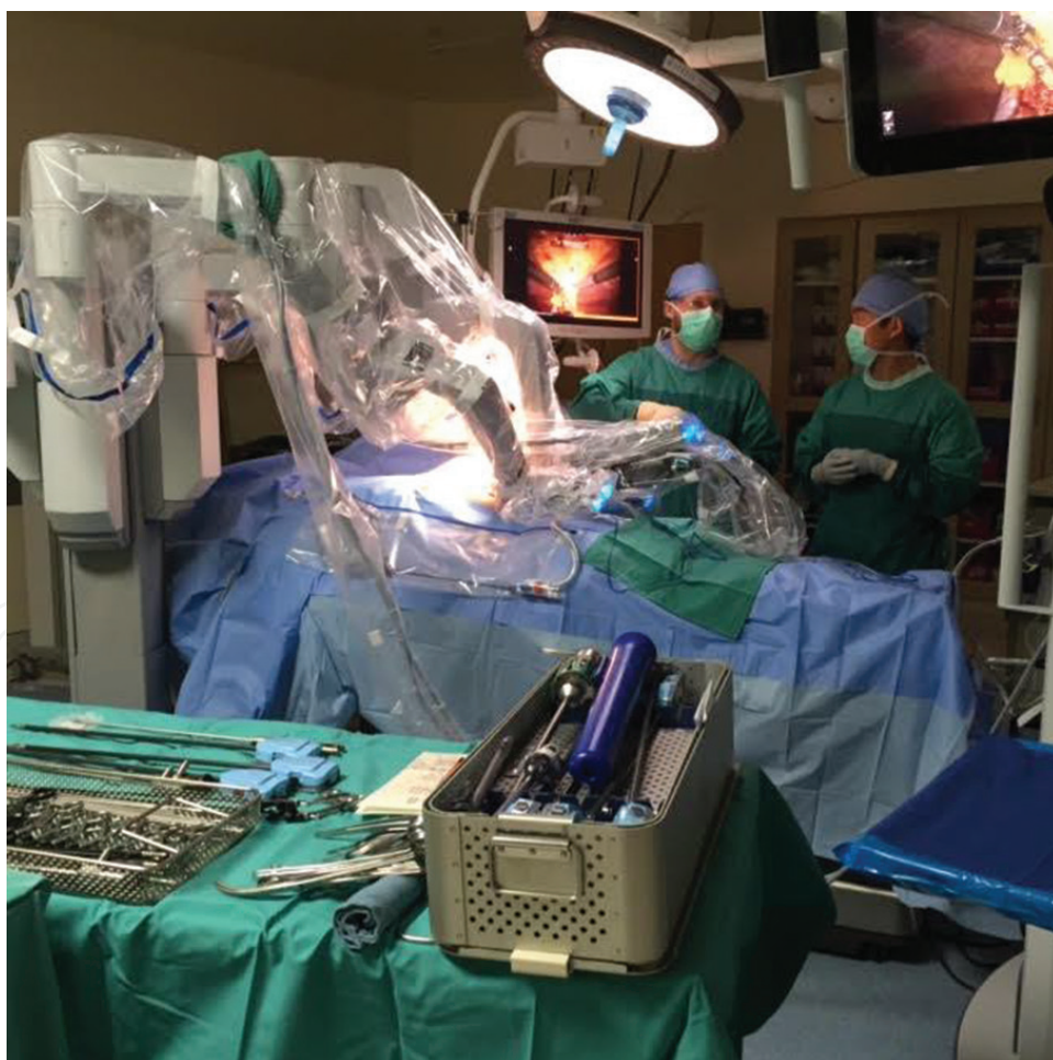
Figure 2. da Vinci system (“slave manipulator”) with robotic arms already docked and executing the tasks with the surgeon in control, with the surgical team at the bedside.
