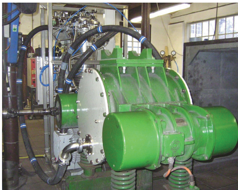
Figure 1. Industrial eccentric vibratory mill (type: ESM 656–0.5 ks, Siebtechnik GmbH, Germany).
