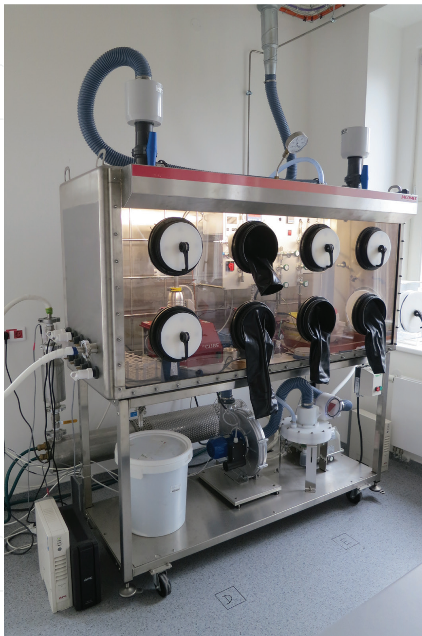
Figure 15. The equipment for safe handling of tritium gas; the tritium manifold (RC-TRITEC AG) placed in the glove box; a scrubber for decontamination placed behind the glove box.
