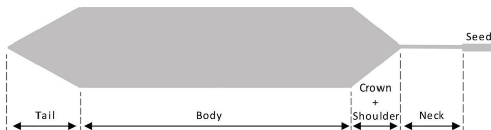
Figure 6. Cross section of a Cz-Si crystal and its different parts after the growth process.
