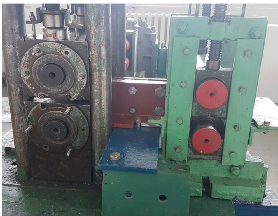
Figure 11. Experimental stand for realization of combined process "rolling-pressing."
