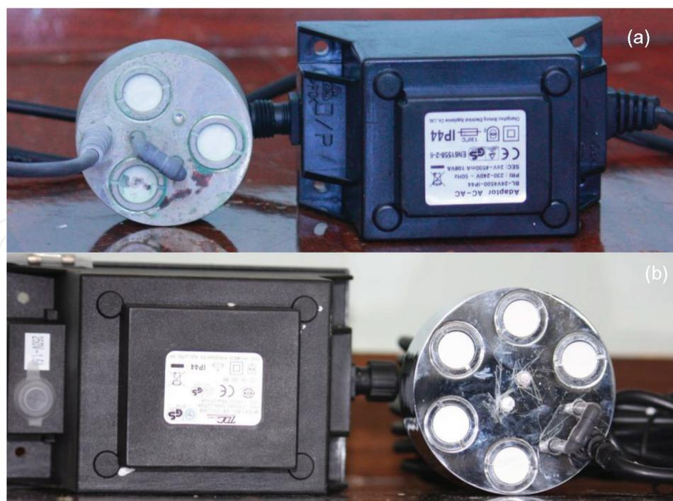
**Figure 7.** Ultrasonic nebulizers employed in the study: (a) shows the 1.7 MHz ultrasonic nebulizer with power supply unit and (b) shows the 4.8 MHz ultrasonic nebulizer with power supply unit.
