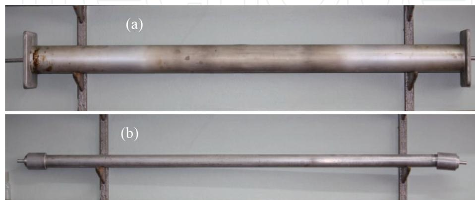
**Figure 10.** The aluminum reaction vessels used for ultrasonic spray pyrolysis deposition of TiO<sub>2</sub> NPs and TFs.
