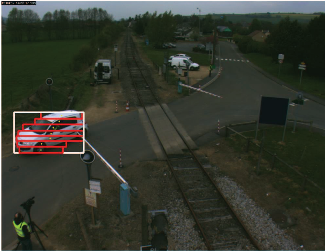
Figure 6. Segmentation of an object using optical flow procedure.
