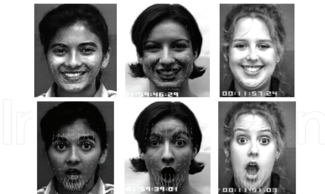
Figure 7. Fitting a deformable face model to images and inferring different facial expressions by taking structural and temporal image features into account
