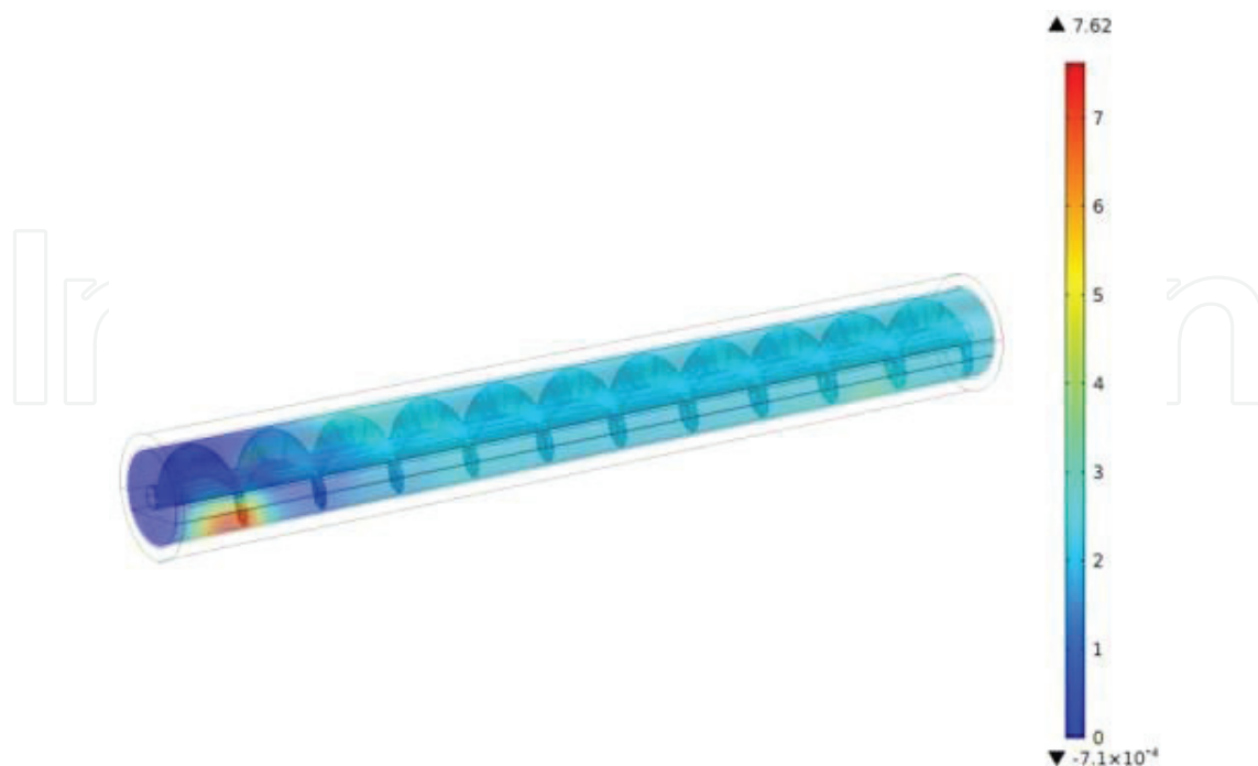
Figure 10. The calculated fields of steam concentrations.
