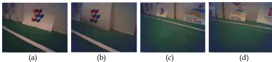
Fig. 1. Examples for finding the best pose in image database. Images in the database are collected in the areas of the field where the robot can not see any landmark every 100mm in x , 100mm in y and 45^\circ in \theta . (a) is the current image taken by robot's camera when its real position is (-1660, 1520, 135^\circ) . (b) is the most similar picture to image (a) in the experience database which the corresponding position of the robot is (-1600, 1500, 135^\circ) . The location error is 60mm in x , 20mm in y , and 0^\circ in \theta . (c) is the random sample image taken after (a) when the real robot position is (-1040, 1220, 135^\circ) . The location error in experience image (d) is 240mm in x , 120mm in y , and 0^\circ in \theta .
