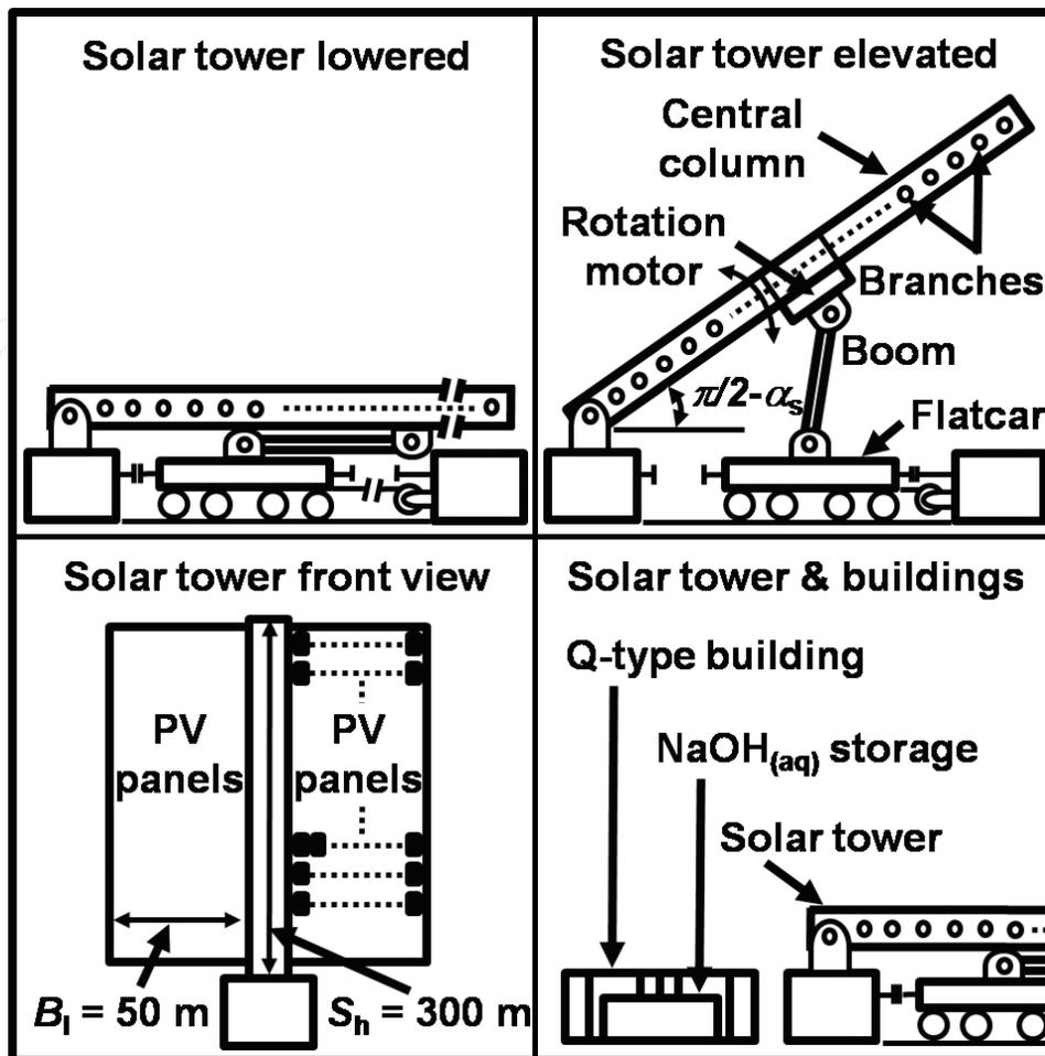
Figure 4. Solar tower architecture (NOT TO SCALE).
