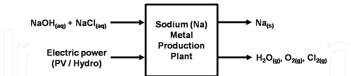
**Figure 1.** Self-contained sodium (Na) metal production plant operating resources diagram.
