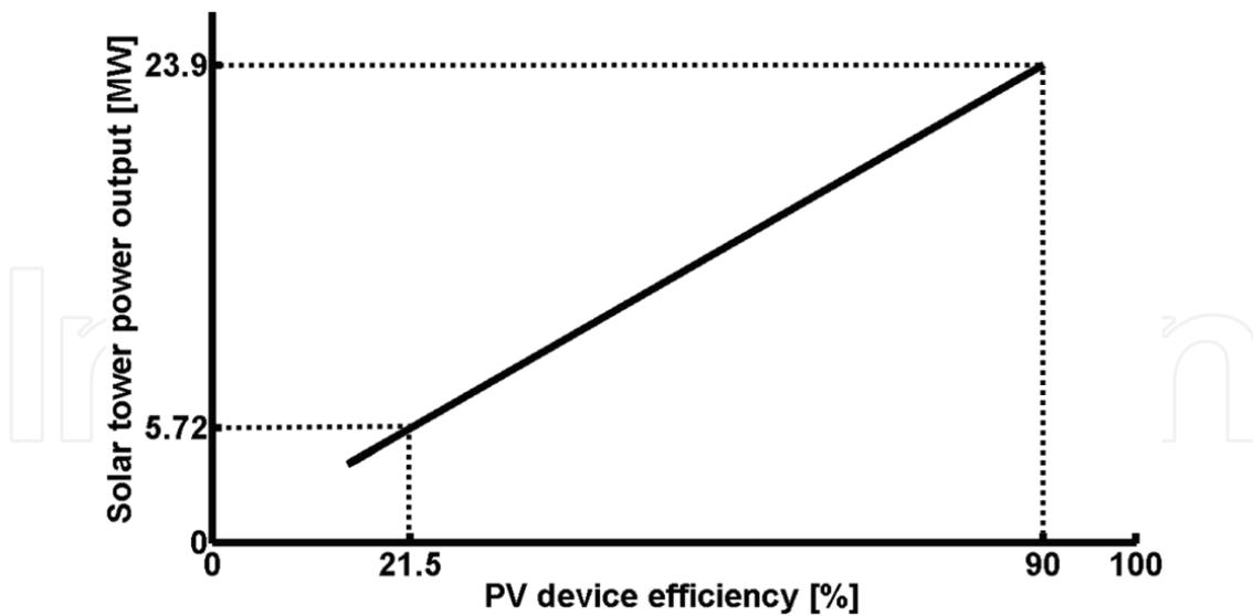
**Figure 3.** Electric power output for a solar tower PV device panel array with area  $A_{PA} = 30,000 \text{ m}^2$  under ASTM direct normal AM 1.5D standard terrestrial solar spectral irradiance as a function of the PV device efficiency.
