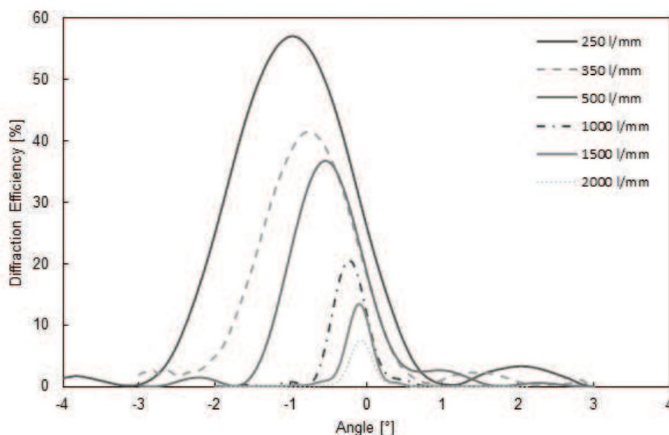
**Figure 16.** Bragg curves (the variation of diffraction efficiency with reading beam angle of incidence) for a series of gratings formed using the single beam process using different spatial frequency seed gratings. Layer thickness is approximately 140  $\mu\text{m}$ .
