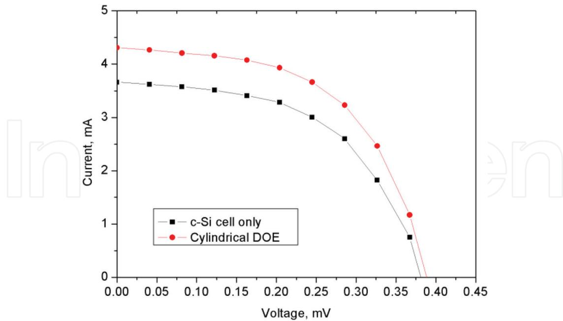
**Figure 6.**  $I$ - $V$  curves for a c-Si solar cell (area = 60 mm<sup>2</sup>) with and without a cylindrical DOE in place.
