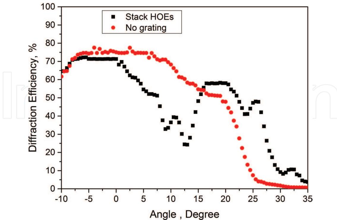
**Figure 5.** The variation of the percentage of light falling on the detector with angle of incidence for a stack of three laminated gratings (from Figure 4) and a clear photopolymer layer with no grating.
