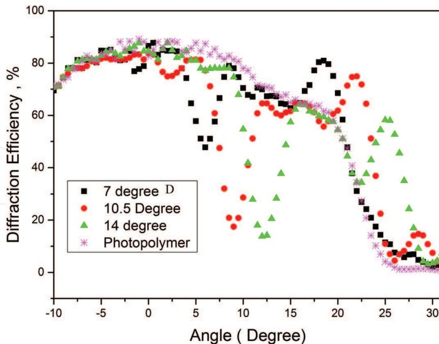
**Figure 4.** The variation of the percentage of light falling on the detector with angle of incidence for three individual gratings recorded at different slant angles with a spatial frequency of 300 lines/mm in layers with thickness of about 50  $\mu\text{m}$ ; the recording intensity was 1  $\text{mW}/\text{cm}^2$ . A photopolymer layer with no grating is included for comparison.
