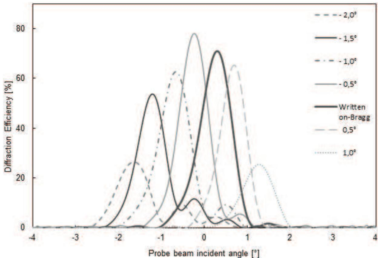
**Figure 14.** Bragg curves (the variation of diffraction efficiency with reading beam angle of incidence) for a series of gratings formed using the single beam process, using different angles of incidence of the single writing beam. The layer thickness is 200  $\mu\text{m}$ . The arrows indicate the offset (in degrees) from the Bragg angle of the seed grating ( $0^\circ$ ).
