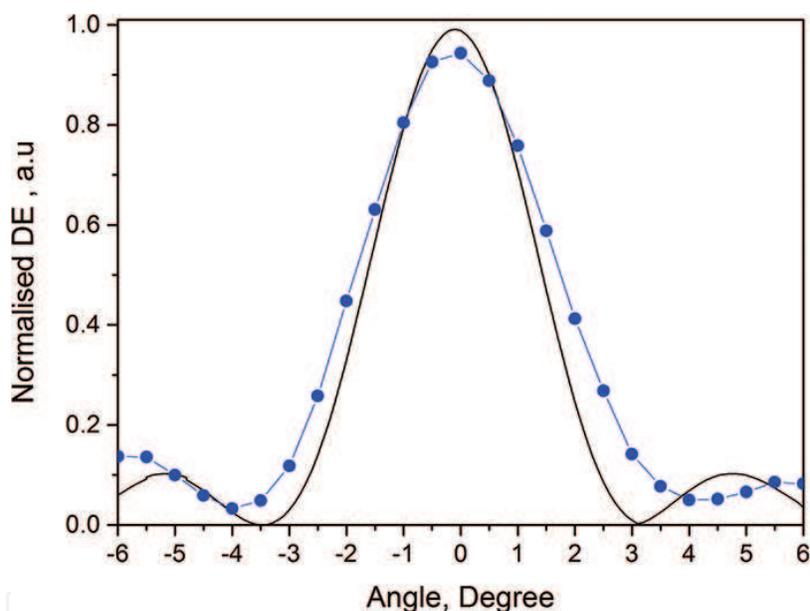
**Figure 3.** Diffraction efficiency versus angle for a cylindrical DOE at central spatial frequency of 300 lines/mm and recording intensity of  $1 \text{ mW/cm}^2$ . The dotted line shows the measured values and the smooth line is the theoretical curve for a 300 lines/mm volume grating of this diffraction efficiency in a 50 micron thick photopolymer layer.
