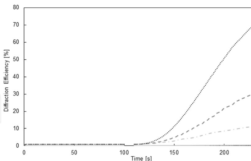
**Figure 15.** Growth in diffraction efficiency, under single beam illumination, of 'seed' gratings in samples prepared with different thicknesses. The grating spatial frequency is 500 lines/mm and the layer thicknesses are approximately 60  $\mu\text{m}$  (solid), 130  $\mu\text{m}$  (dotted-line), 190  $\mu\text{m}$  (dashed line) and 240  $\mu\text{m}$  (dotted line). Initial diffraction efficiency is approximately 1% for the two-beam grating.
