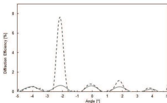
**Figure 17.** Variation of diffraction efficiency with the reading beam angle of incidence for a series of gratings, from which one individual grating has been enhanced by illuminating with a single on-Bragg beam of light. The angular separation between neighbouring gratings is  $2^\circ$ .
