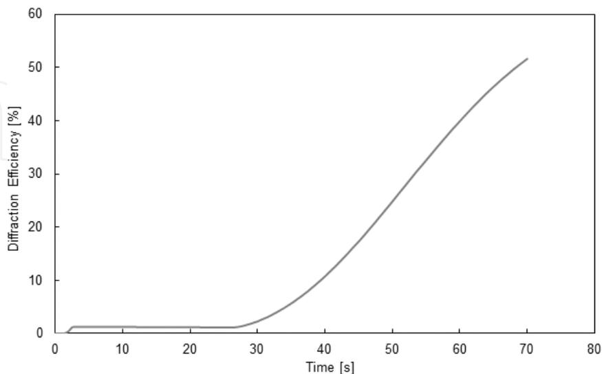
**Figure 13.** Diffraction efficiency versus exposure time. A standard two-beam holographic recording of 2 sec is followed by a 25 sec delay (no illumination) and then illumination with just one of the writing beams. Exposure intensity is 2.5  $\text{mW}/\text{cm}^2$  in each beam.
