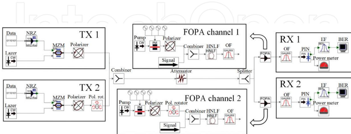
**Figure 21.** Simulation model of the two-channel optical transmission system with FOPA for division and amplification of polarization-multiplexed signals.
