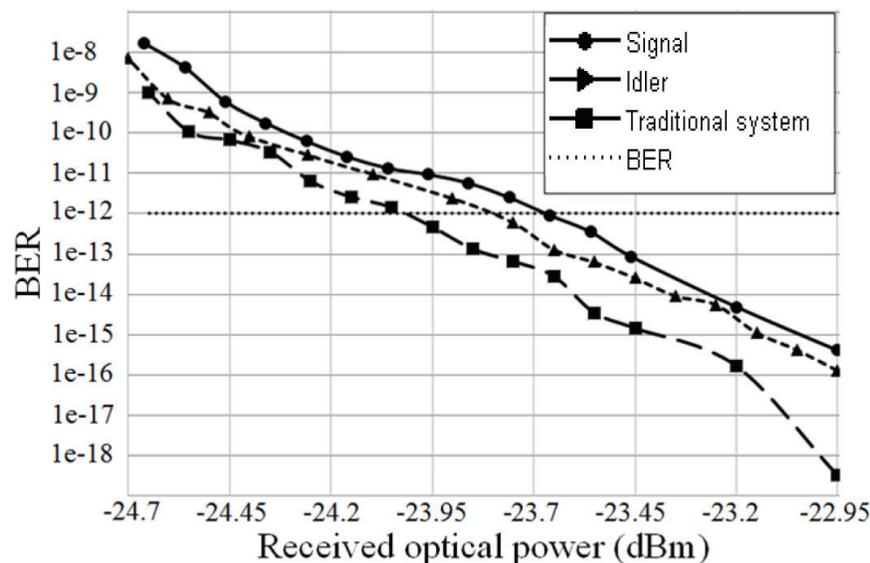
**Figure 17.** BER value dependence on the detected signal power in the standard single-channel transmission system (dashed line) and in the system with modulation format conversion at the initial signal frequency (solid line) and at idler frequency (dotted line).
