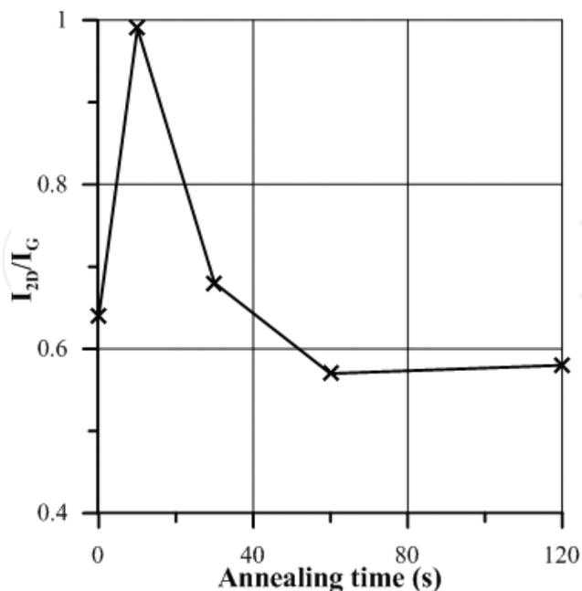
**Figure 8.** Ratio of 2D and G band intensities in Raman spectra of graphene prepared by annealing at 850°C and at various times. (Reprinted with permission from Applied Surface Science No. 3995260811830.).
