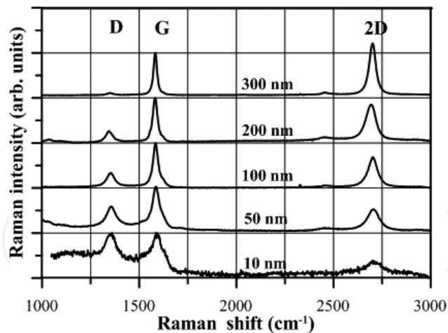
**Figure 5.** Raman spectra of several Co/SiC structures differing in Co layer thickness. (Reprinted with permission from J Mater Sci: Mater Electron, No. 3995250684677.).
