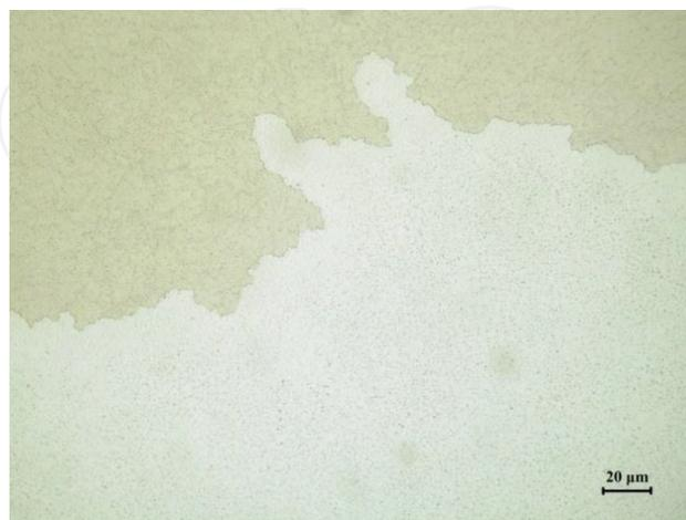
**Figure 6.** Example of a structure surface with Co layer 300 nm thick annealed at 990°C for 60 s. (Reprinted with permission from J Mater Sci: Mater Electron, No. 3995250684677.).
