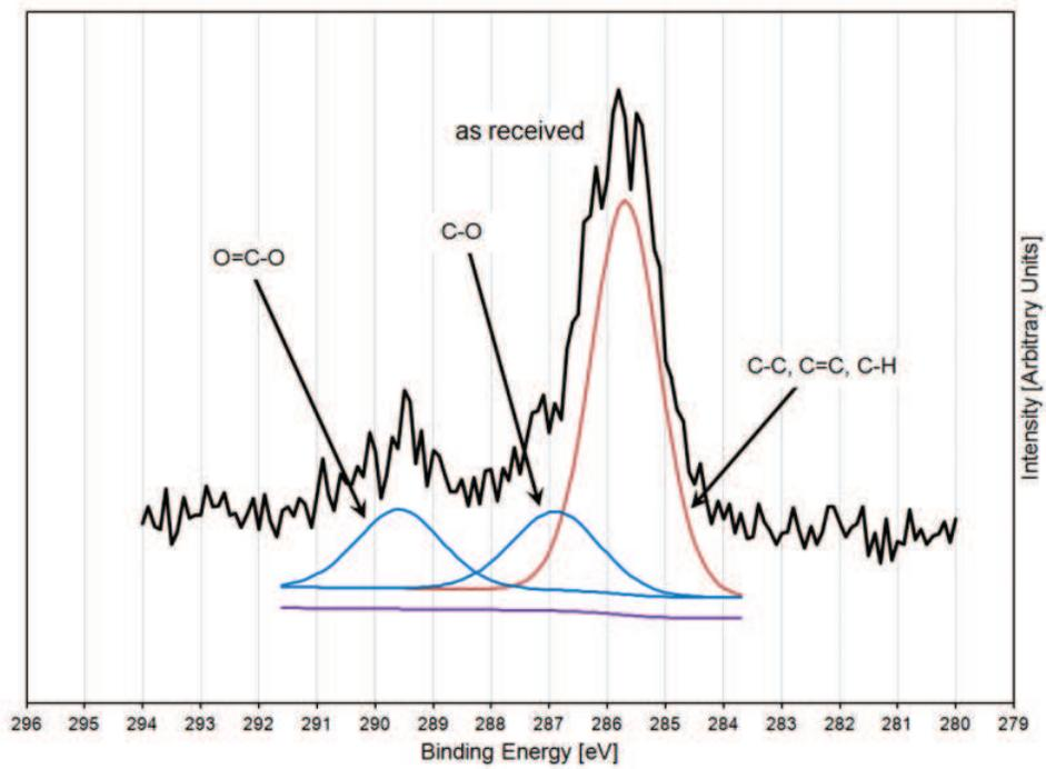
**Figure 14.** Fitted C 1s peak of the as-received sample. For clarity, peak components and background are vertically slightly offset. (Reprinted with permission from Thin Solid Films No. 3995281012757.).
