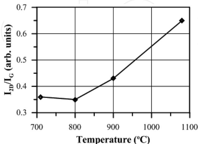
**Figure 2.** Ratio of 2D and G band intensities in Raman spectra of graphene on the Ni(200)/SiC structures annealed at various temperatures. (Reprinted with permission from Thin Solid Films No. 3995281012757.).
