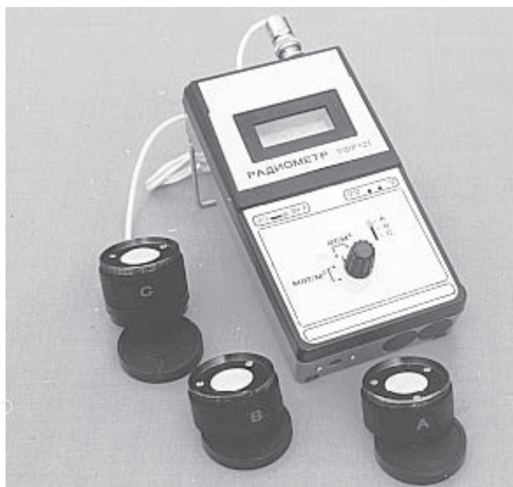
Figure 10. A handheld UV radiant power meter UVR-21 with FTO-GaP-based radiometric heads.
