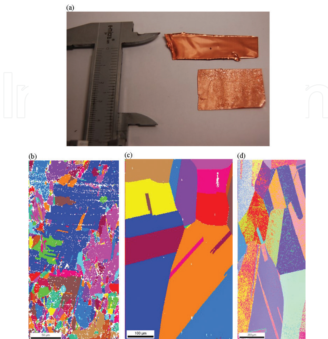
Figure 5. (a) Polycrystalline copper foil before (up piece) and after (down piece) the hydrogen etching. The difference in the surface colour indicates the deoxidation of it. The red line indicates 4 cm. EBSD maps of (b) the as-received polycrystalline copper foil (scale bar 50 \mu\text{m} ), (c) the foil after plasma annealing and 20 min graphene growth at 1040°C (scale bar 100 \mu\text{m} ), and (d) the foil after plasma annealing and 50 min graphene growth (scale bar 200 \mu\text{m} ).
