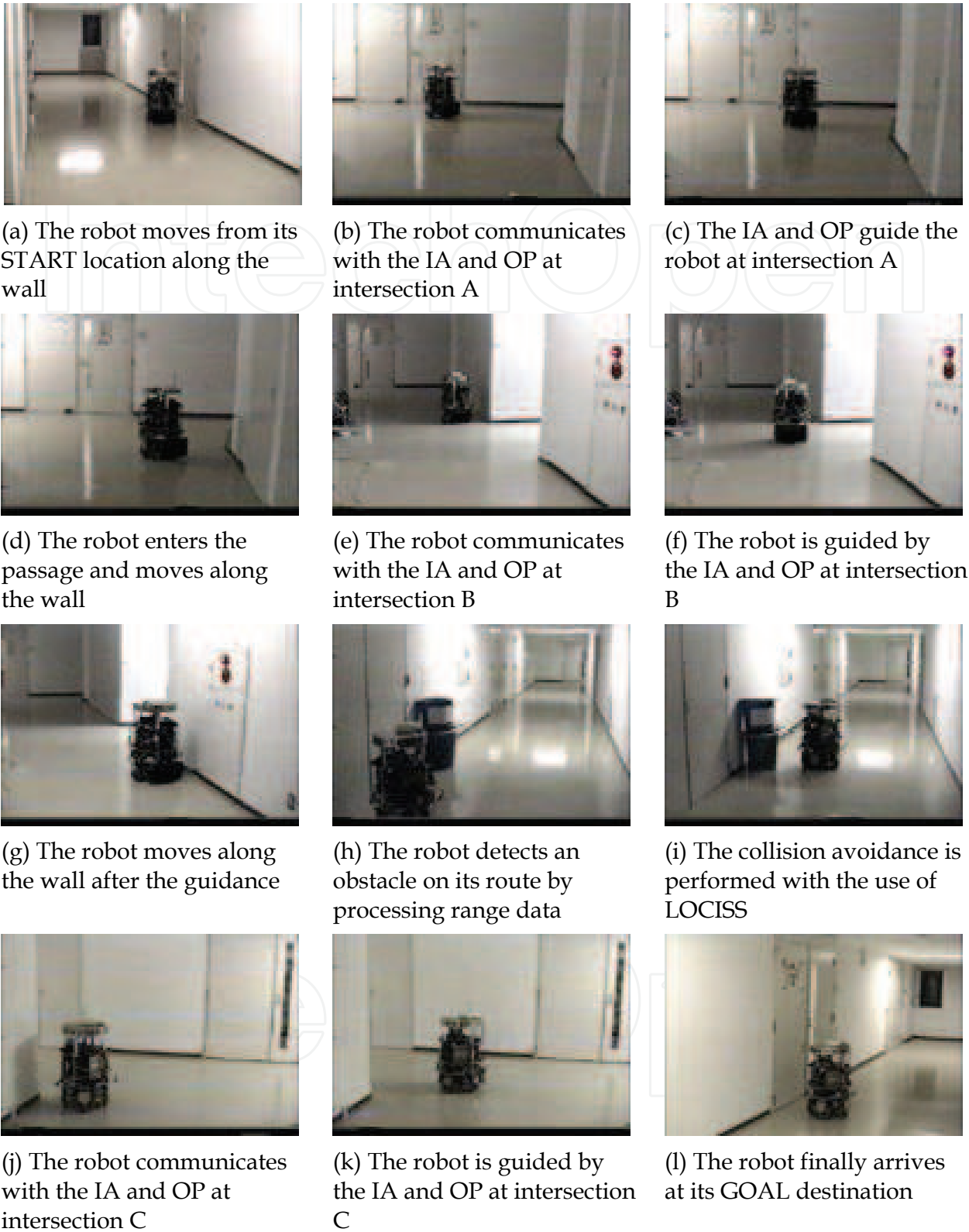
Figure 12. Robot navigation experiment with the IA and OP devices
