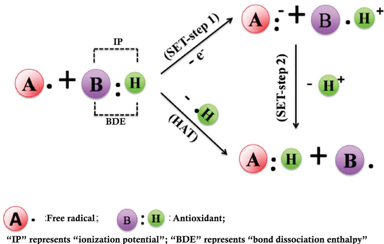
**Figure 2.** Reaction mechanisms of single-electron transfer (SET) and hydrogen atom transfer (HAT) [16]. Both mechanisms almost always occur together in all samples, with the balance determined by antioxidant structure and pH.
