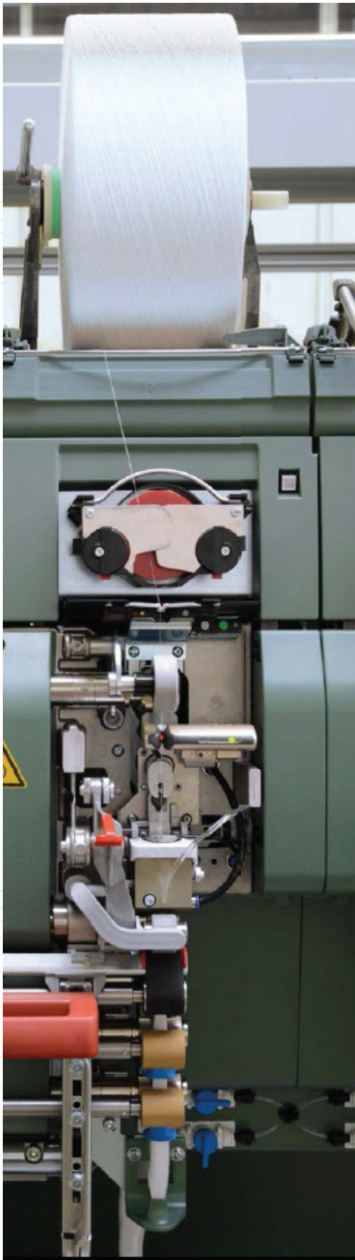
Figure 13. Rieter automated air-jet spinning machine [27].
