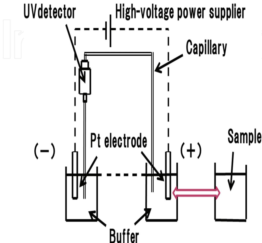
Figure 6. Illustration of a laboratory-built CE instrument.
