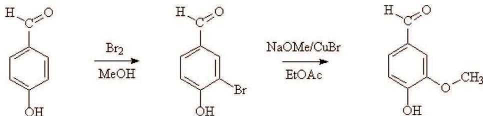
**Figure 2.** Laboratory synthesis scheme of vanillin.
