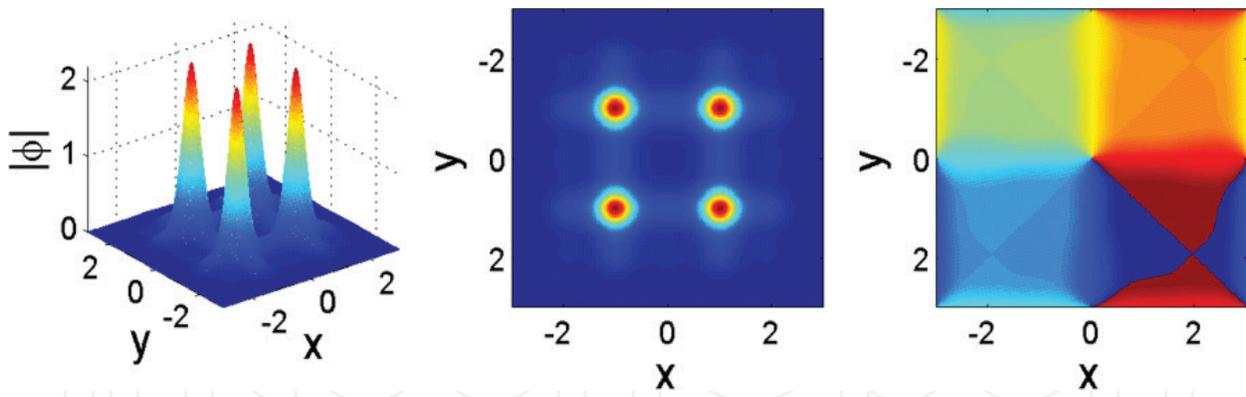
**Figure 15.** Shape of a stable vortex with topological charge 1 inside the semi-infinite gap supported by the full 2D linear and nonlinear potentials, for  $q = 1$  and  $g = +1$ . The left, middle to right panels show, respectively, the absolute value of the field,  $|\varphi(x, y)|$ , in cylindrical coordinates and its contour plot, as well as the phase distribution that carries the vorticity. Parameters of the vortex are  $\mu = -5.1$  and  $N = 4.4$ .
