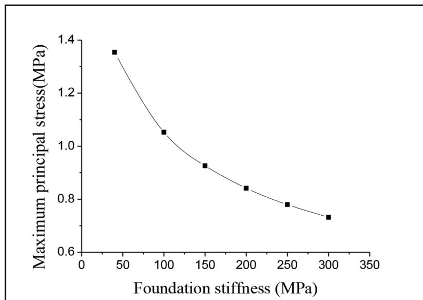
**Figure 3.** Relation curve of maximum principal stress and foundation stiffness.
