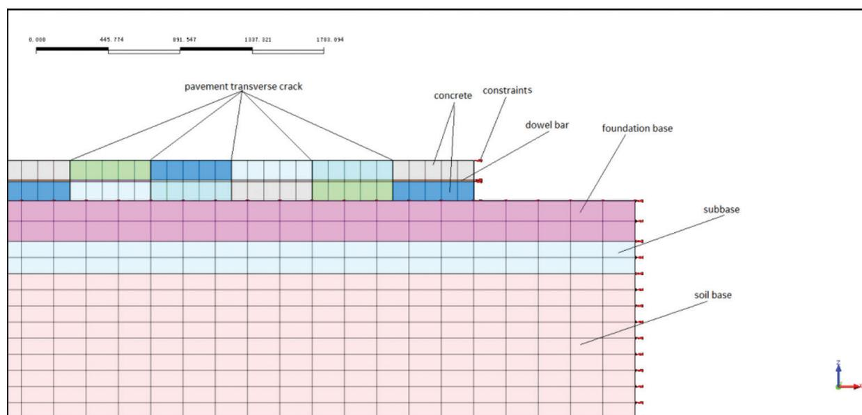
**Figure 1.** Schematic diagram of pavement structure.
