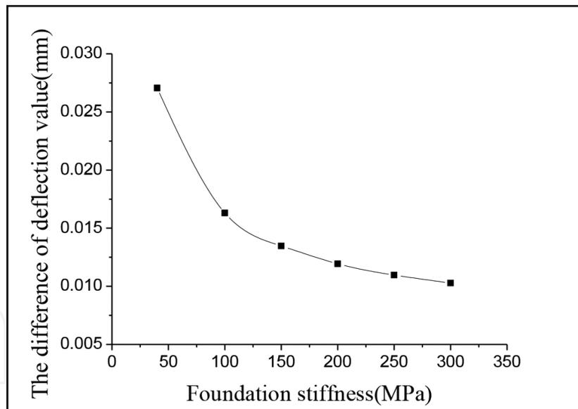
**Figure 2.** Relationship between the top deflection of the plate and the foundation stiffness.
