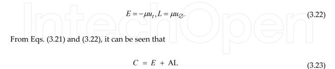
which shows that the linear combination of energy and angular momentum is constant along a streamline but varies from streamline to streamline. Thus, *C* is a streamline invariant.
