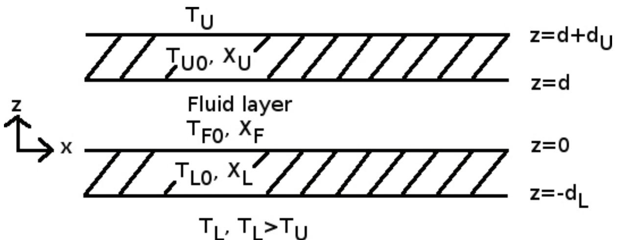
**Figure 1.** Scheme for the problem of Rayleigh convection including the thickness and thermal conductivities of the walls.  $T_{L,U}$  stand for the constant temperature at the lower and upper walls,  $T_{L0,U0,F0}$  stand for the basic state temperature profile at the lower wall, upper wall and fluid layer; while  $X_{L,U,F}$  represent the thermal conductivities of the lower wall, upper wall and fluid layer, respectively. Dimensional variables are used.
