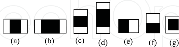
Fig. 5. (a), (b) and (c) are templates for line features; (e) and (f) are for edge features and (g) is the center-surrounded feature
