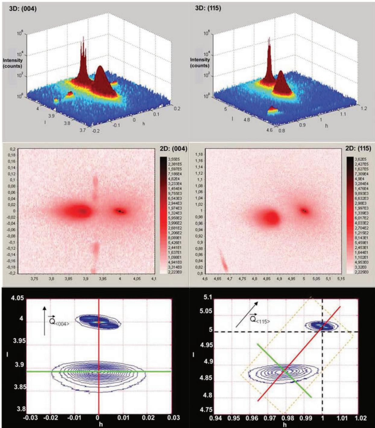
**Figure 13.** 3D and 2D reciprocal space maps of  $\text{In}_{0.08}\text{Ga}_{0.92}\text{As}/\text{GaAs}$  structure, recorded around (004) and (115) nodes. In the bottom, contour curves of iso-intensity are drawn. Diffusion vectors  $\vec{Q}_{(004)}$  and  $\vec{Q}_{(115)}$  were added to corresponding RSM.
