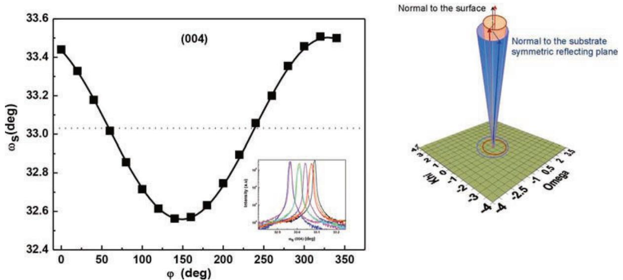
**Figure 2.** In the left, measured Bragg angle GaAs substrate of (004) rocking curves as a function of the azimuthal angle  $\varphi$  fitted by (the solid line) a sinusoidal equation. In the inset a series of rocking curves are shown. In the right, illustration of  $\omega$ -scan around the normal to the substrate.
