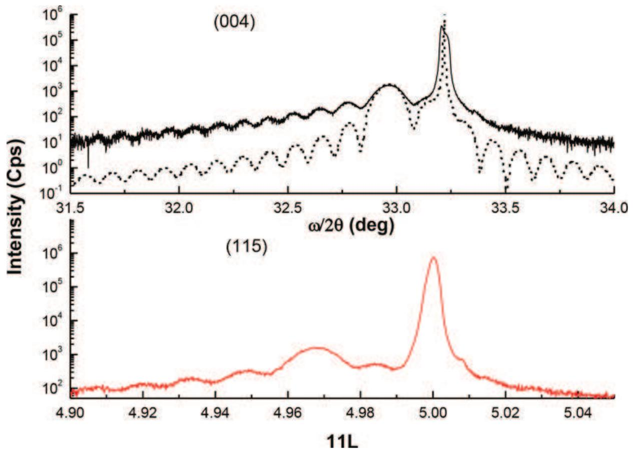
**Figure 9.** In the top: HRXRD (004) experimental  $\omega/2\theta$  curve (solid line) and simulated curve (dotted line) of GaAs<sub>0.963</sub>Bi<sub>0.37</sub> layer grown on (100) Zn doped GaAs substrate. In the bottom: optimized scan of HRXRD (11L) reflection plane. L is changed around 5.
