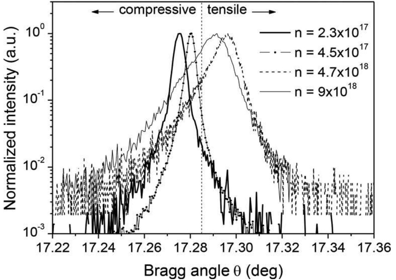
Figure 5.  $\omega$ -scans of the Si-doped GaN samples.
