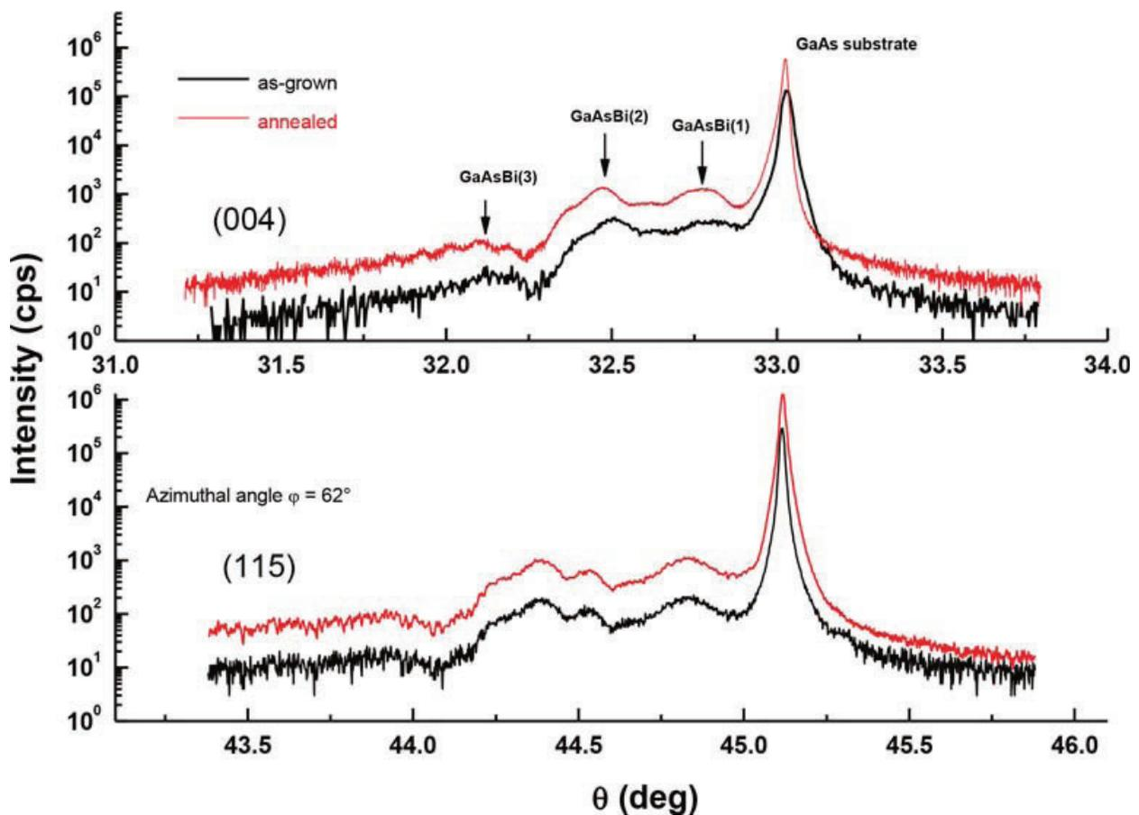
**Figure 10.** HRXRD (004) and (115) experimental  $\omega/2\theta$  patterns of as-grown and annealed GaAsBi layers grown on GaAs substrate at  $420^\circ\text{C}$  under  $3 \mu\text{mol min}^{-1}$  of TMBi flow.
