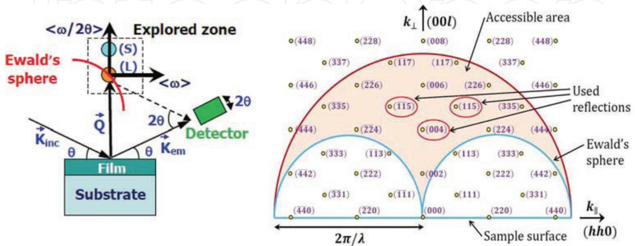
**Figure 12.** Ewald construction illustrating the scattering geometry in the cases of symmetrical and asymmetrical reflexes. The grey arrows show the scan directions for  $\omega/2\theta$ -scan and a  $\omega$ -scan. The accessible reflections in conventional scattering geometry are shown.
