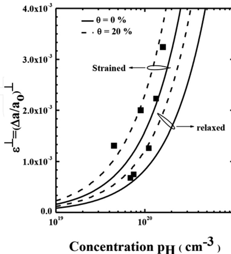
**Figure 3.** Perpendicular lattice mismatch ( $\epsilon^\perp$ ) of GaAs:C epilayers on GaAs substrates as a function of hole concentration  $p_H$ . The lines represent the predicted contraction based on Vegard's law for two values of compensation ratios  $\theta = 0$  and  $\theta = 0.25$ .
