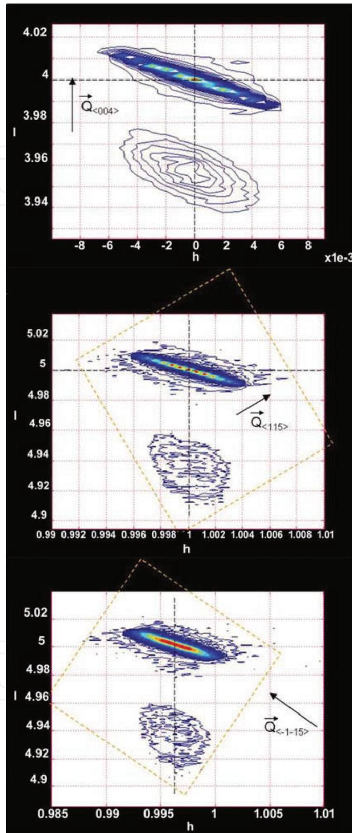
**Figure 14.** Reciprocal space mapping of  $\text{In}_{0.08}\text{Ga}_{0.92}\text{As}/\text{GaAs}$  structure, recorded around (004), (115) and  $(\overline{1}\overline{1}\overline{5})$  nodes. Diffusion vector  $\vec{Q}_{(hkl)}$  was added to the corresponding RSM.
