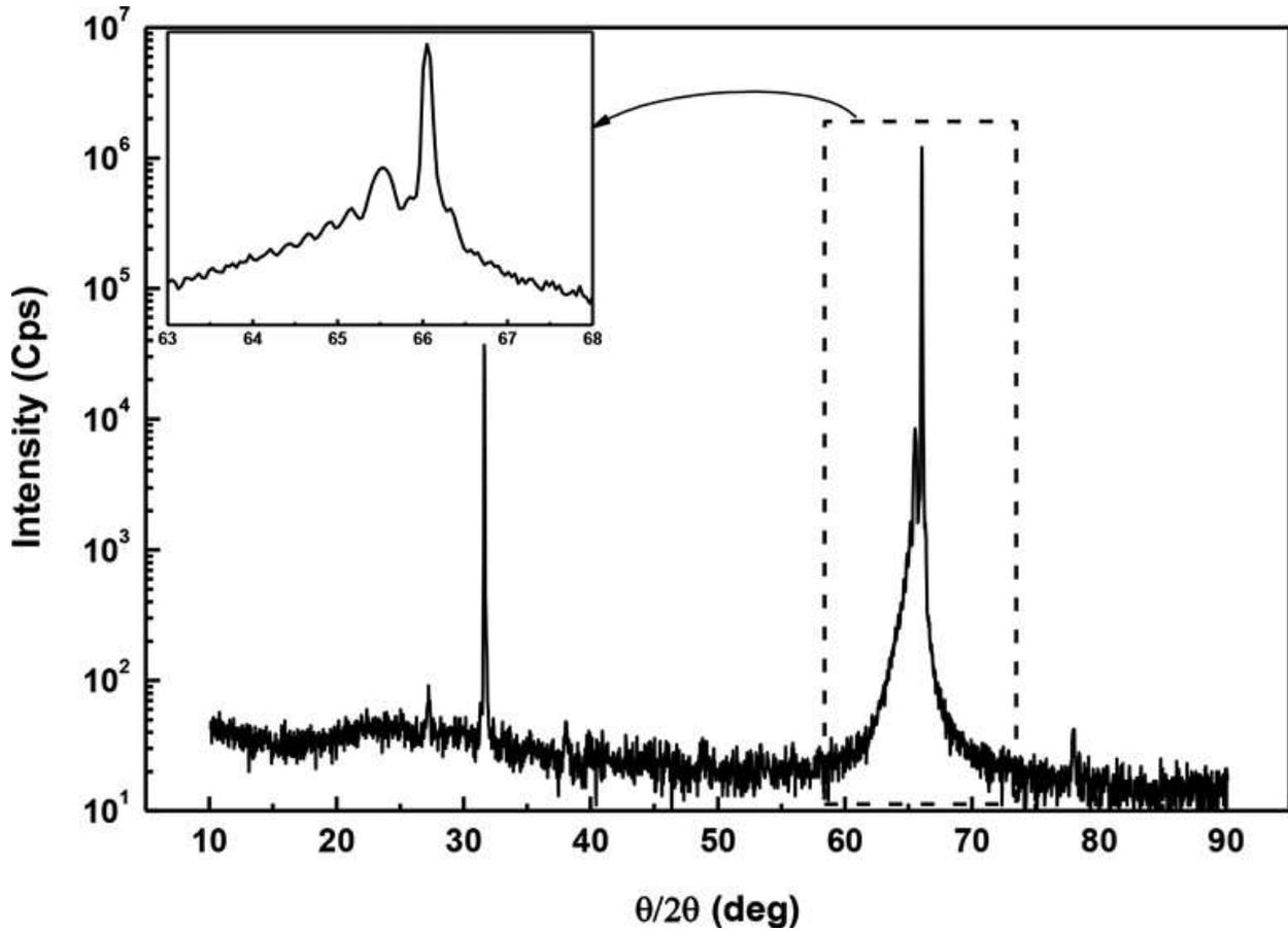
**Figure 8.** Diffraction pattern in the  $\theta-2\theta$  scan of X-ray diffraction measurement for a  $\text{GaAs}_{1-x}\text{Bi}_x$  layer grown on (100) Zn doped GaAs substrate. The inset shows a zoom between  $2\theta = 63^\circ$  and  $68^\circ$ .
