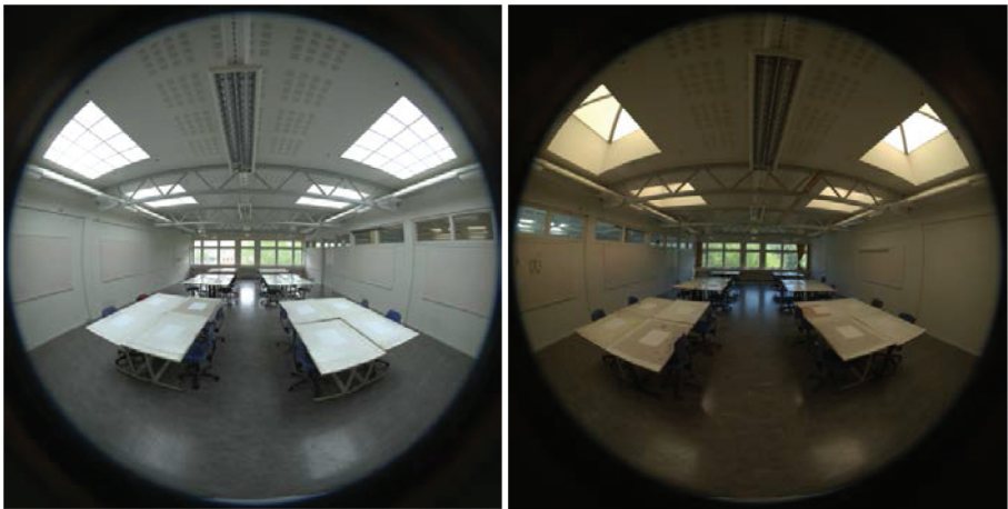
Figure 7. Fish eye HDR pictures of the studio under overcast sky conditions, the new solution to the left, old one to the right.
