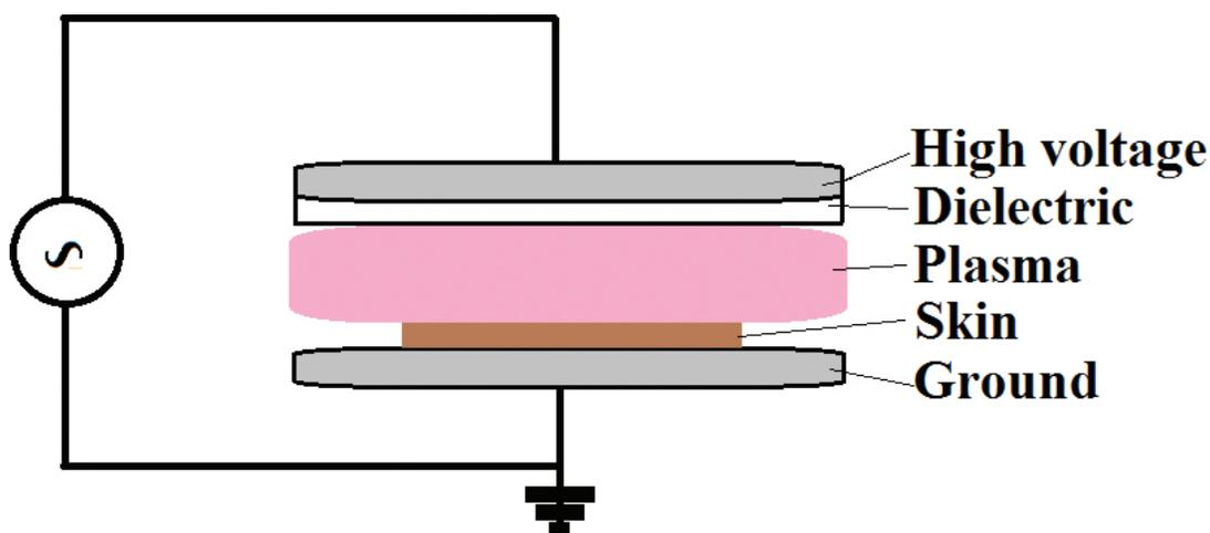
**Figure 4.** Volume dielectric barrier discharge.
