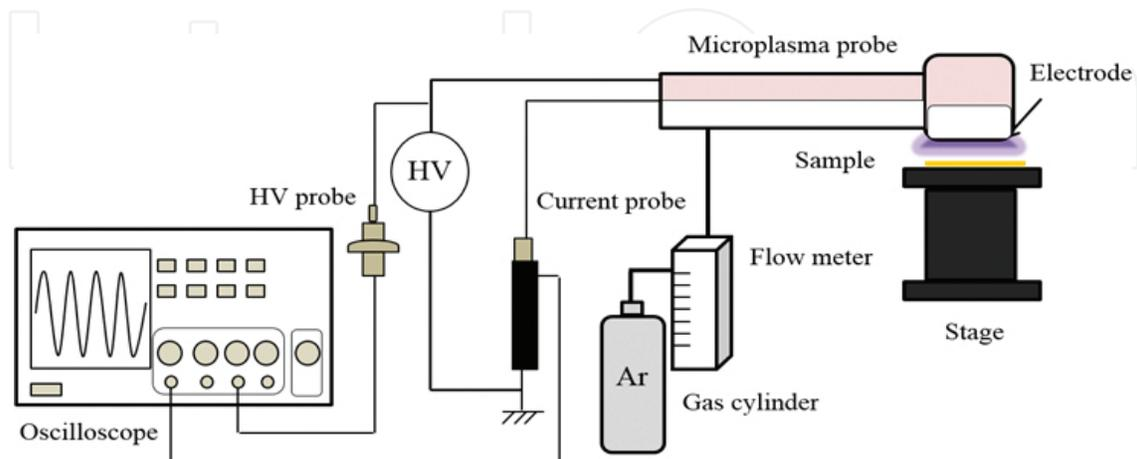
Figure 7. Experimental set-up with microplasma electrode [23].
