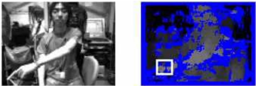
Fig. 8. Pointing gesture recognition based on depth image
