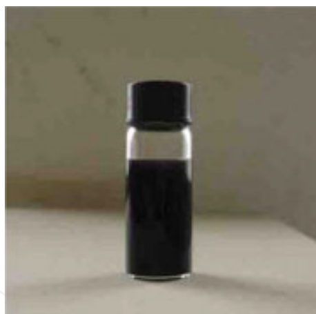
Figure 4. Picture of the nickel nanoparticles in PAO6 after a month.
