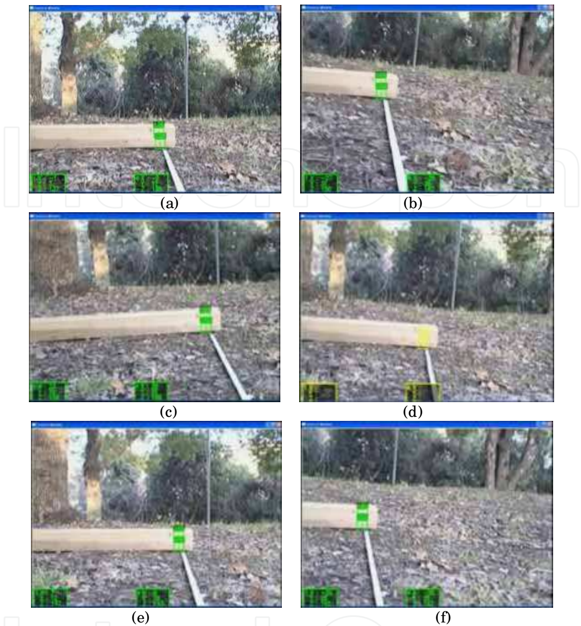
Fig. 14. Execution results of the proposed algorithm for simultaneous execution of the tracking and the stereo matching. Two small windows at the center part of images are shown the tracking windows, and the windows at the bottom of the images are shown parameters of the tracking points. The target points were not lost though the camera system was intensely shaken for five seconds. Although the stereo matching failed on two frames (the color of target window changed to yellow as shown in (d)), the distance measurement succeeded in almost all frames.
