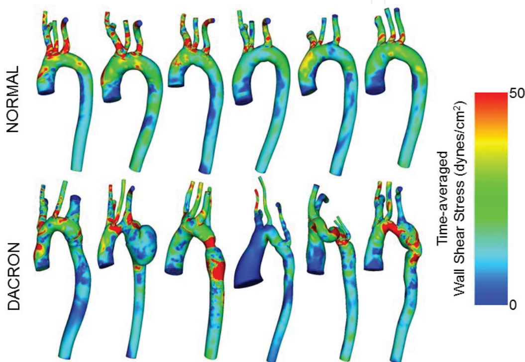
Figure 10. CFD for arch repair by Dacron patch. Time-averaged WSS distributions in six normal subjects (top, 5M, 1F ages 25–33 years) as well as age- and gender-matched patients previously treated for CoA by Dacron patch aortoplasty (below).
