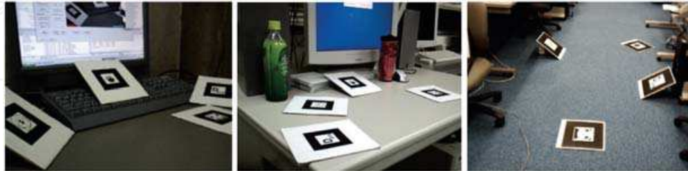
Fig. 7. Object scenes where multiple markers are distributed at arbitrary positions and poses
