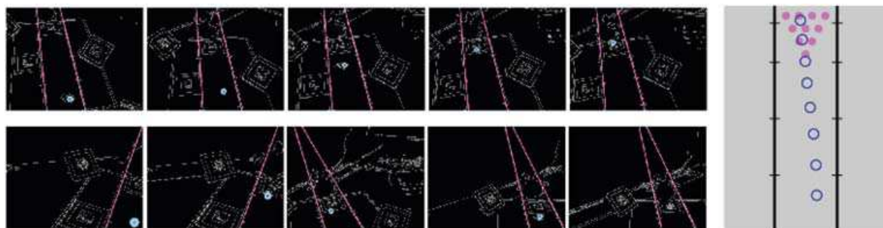
Fig. 26. Detected lane and ball, and trajectory of ball
