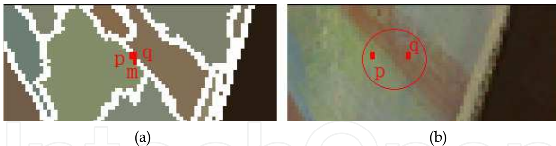
Fig. 16. (a): position relation illustration of pixels on region boundary(part magnified image of Fig.15(b)); (b): principle of region boundary pixels matching illustration(part magnified image of Fig.15(c))
