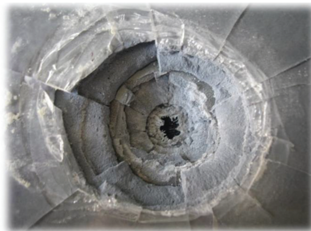
Figure 13. Crater originated in the double ceramic plate.
