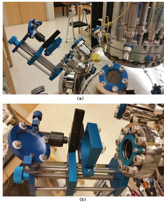
**Figure 2.** View of the 24" vacuum chamber of the three-beam MBMT-MAPLE/PLD system at Dillard University (a). The side view of one of the laser beam guides including the holder for the laser beam scanner attached to the optical window of the chamber (b) [60].
