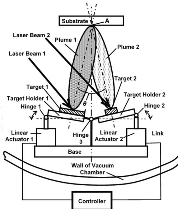
**Figure 3.** Schematic of the target tilting sub-system of the MBMT-MAPLE/PLD system with remote control of the directions of the plumes. Shown are two targets out of three.  $\theta$  is the optimal angle between the plumes at which they overlap in point A on the surface of the substrate.
