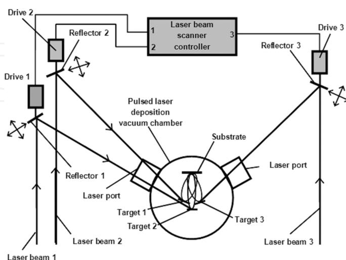
**Figure 1.** The schematic of the MBMT-MAPLE/PLD system [60].
