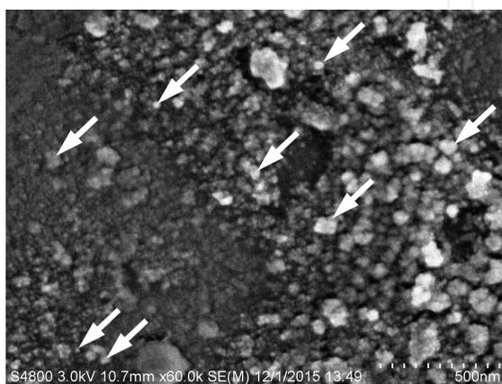
**Figure 12.** Scanning electron microscopy (SEM) image of the three-component composite film made of PMMA and the nanoparticles of  $\text{NaYF}_4: \text{Yb}^{3+}, \text{Er}^{3+}$  and AZO taken with magnification  $\times 60,000$ . White arrows point to exemplary nanoparticles of various sizes (from  $\sim 10$  to 200 nm) embedded in the polymer matrix.
