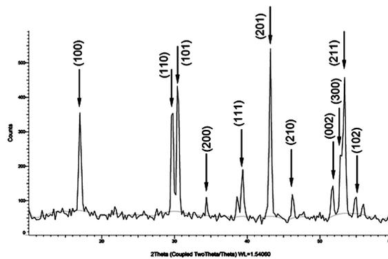
**Figure 10.** XRD spectrum of the two-component composite film made of PMMA and the nanoparticles of  $\text{NaYF}_4$ :  $\text{Yb}^{3+}$ ,  $\text{Er}^{3+}$  with the diffraction peaks attributed to the hexagonal  $\beta$ -phase of  $\text{NaYF}_4$ .
