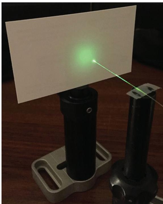
**Figure 14.** Photograph of the tip of a single-mode fiber coated with a nano-composite film of PMMA + NaYF<sub>4</sub>: Yb<sup>3+</sup>, Er<sup>3+</sup> + AZO pumped with a 980-nm laser diode (125-mW power) illuminating white back side of a business card.
