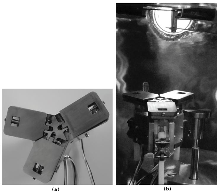
**Figure 4.** View of the three-target holder with remotely controlled tilt of each target (to achieve overlapping of the plumes on the substrate) (a) and the view of the three-target holder installed inside the vacuum chamber (b).
