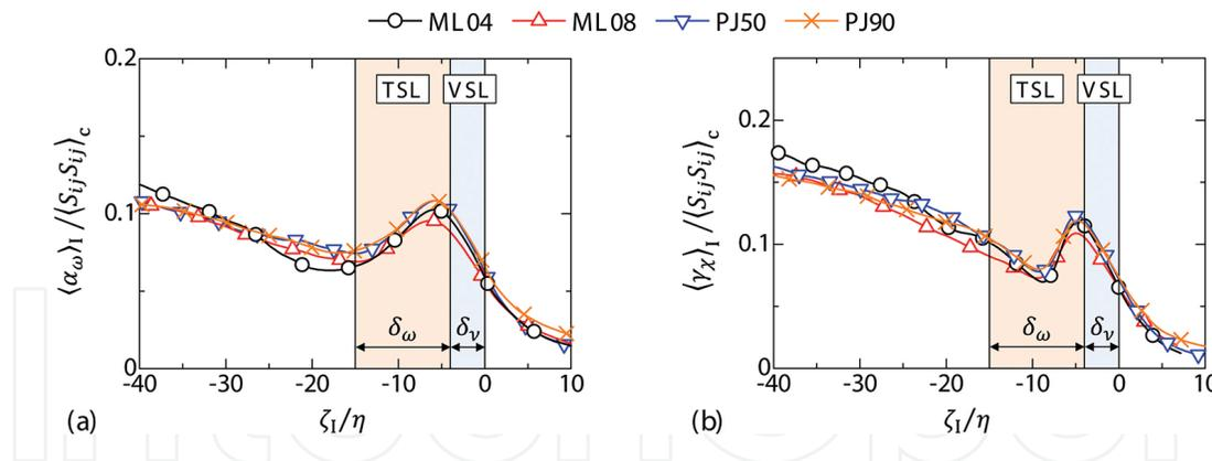
**Figure 8.** Conditional mean profiles of (a) effective extensive strain acting on vorticity  $\alpha_\omega = \omega_i S_{ij} \omega_j / (\omega_k \omega_k)$  and (b) effective compressive strain acting on scalar gradient  $\gamma_\chi = -G_i S_{ij} G_j / (G_k G_k)$ , where the mean strain product on the centerline  $\langle S_{ij} S_{ij} \rangle_c$  is used for normalization. The viscous superlayer and turbulent sublayer are also indicated.
