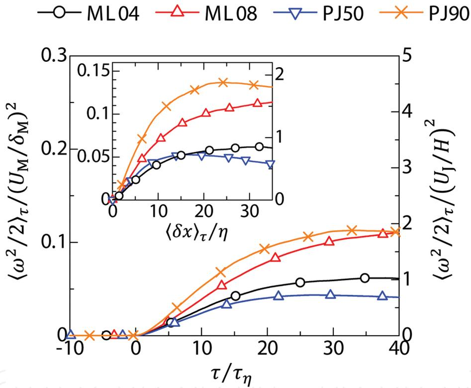
**Figure 11.** Lagrangian conditional mean enstrophy  $\langle \omega^2/2 \rangle_\tau$ . The inset plots  $\langle \omega^2/2 \rangle_\tau$  against the mean distance between the particle and the irrotational boundary.
