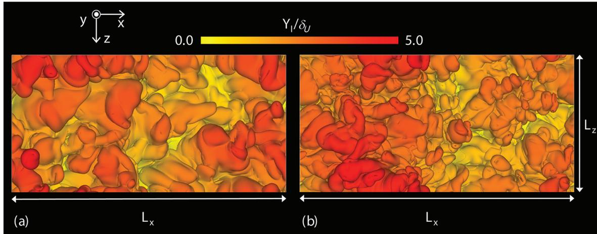
**Figure 4.** Visualization of the irrotational boundary (the vorticity magnitude isosurface) in the mixing layers with (a) Re = 400 and (b) Re = 800. The color shows the interface height  $Y_1$  from the centerline normalized by the mixing layer thickness  $\delta_U = \int (0.5U_M - \langle U \rangle)(\langle U \rangle - 0.5U_M)/(U_M)^2 dy$ .
