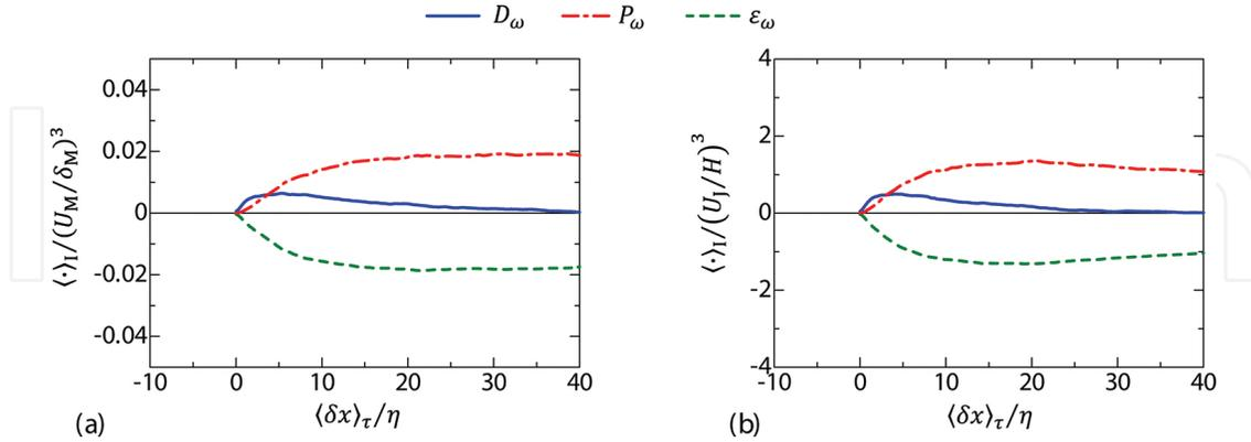
**Figure 12.** Lagrangian conditional mean entrophy budget of the entrained particles plotted against the mean distance  $\langle \delta x \rangle_\tau$  between the particle and the irrotational boundary. (a) ML08 and (b) PJ90.
