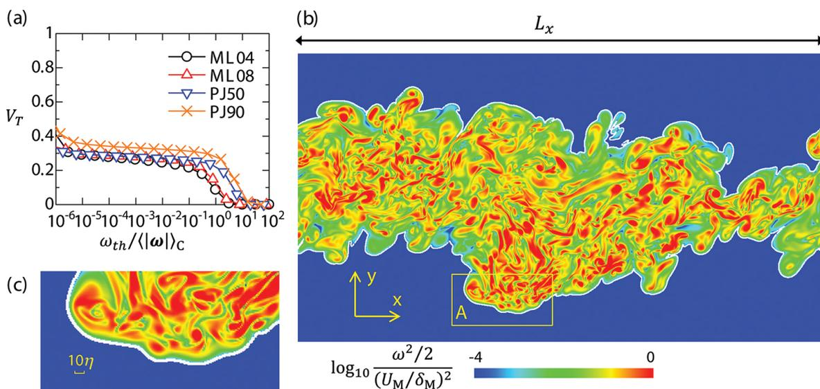
**Figure 3.** Detection of the T/NT interface. (a) Dependence of the turbulent volume fraction on the normalized threshold  $\omega_{th}/\langle|\omega|\rangle_C$ . (b) Visualization of the irrotational boundary in ML08 (white line). The color contours show enstrophy levels in  $\log_{10}(\omega^2/2)$ . (c) The close-up of the T/NT interface (the region A in (b)).
