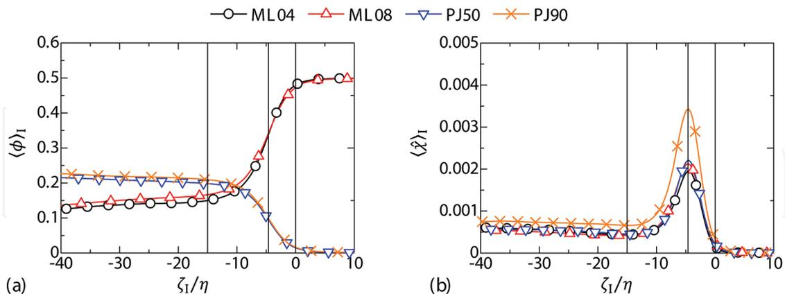
**Figure 7.** Conditional mean scalar ( $\phi$ ) and normalized scalar dissipation rate ( $\hat{\chi}$ ), where  $\hat{\chi} = (\delta_M^2 / ReSc)\nabla\phi \cdot \nabla\phi$  in the mixing layers and  $\hat{\chi} = (H^2 / ReSc)\nabla\phi \cdot \nabla\phi$  in the planar jets. The vertical lines, from right to left, denote  $\zeta_1 = 0$ ,  $\zeta_1 = -4.9\eta$ , where  $\langle \hat{\chi} \rangle_1$  reaches a peak, and  $\zeta_1 = -15\eta$ .
