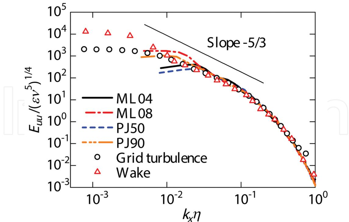
**Figure 2.** One-dimensional longitudinal spectrum  $E_{uu}$  on the centerline of the planar jets and mixing layers compared with the experimental plots in grid turbulence [25] and axisymmetric wake [26].
